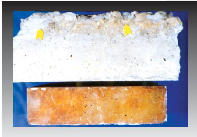
Fig. 1. Concrete beam (top) after 16 years outdoor exposure to a severe sulfate environment, with its upper surface deteriorated. Companion concrete prism (bottom) continuously immersed in a similar solution in a laboratory shows no deterioration. (68854)
