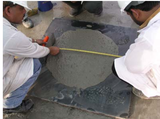
Figure 10 – SCC Conc. Flow Table Testing
