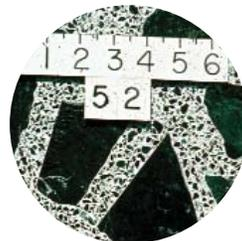
**Panel 52:** Broken pieces of marble tile were adhered to the form face and surrounded by mortar. Following aging for 60 days, the surface was ground and polished. (IMG13773)
