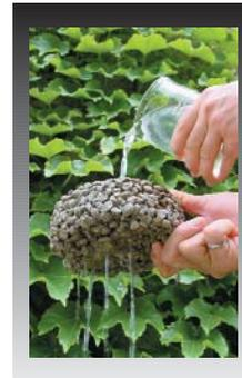
**Figure 1. Pervious concrete uses conventional concrete materials, but the coarse aggregate is kept within a narrow grading and little to no fine aggregate is used. The paste content is also tightly controlled to provide a concrete with an open, porous structure and a high water flow capacity. Photo courtesy of CTL.**
