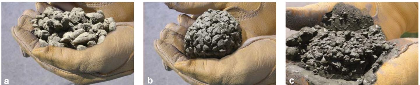
**Figure 2. Samples of pervious concrete with different water contents formed into a ball: (a) too little water, (b) proper amount of water, (c) too much water. [IMG15595, IMG15596, IMG15597]**
