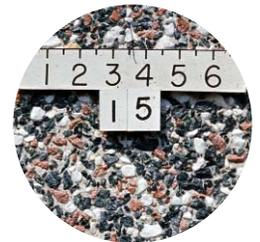
**Panel 15:** Three aggregates in three colors—dark green, white, and pink—are combined for another exposed aggregate surface. (IMG13745)
