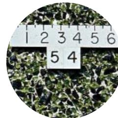
**Panel 54:** Special (non-reactive) green glass used in two sizes gives a green-and-black effect. This panel also has excellent color retention. (IMG13774)
