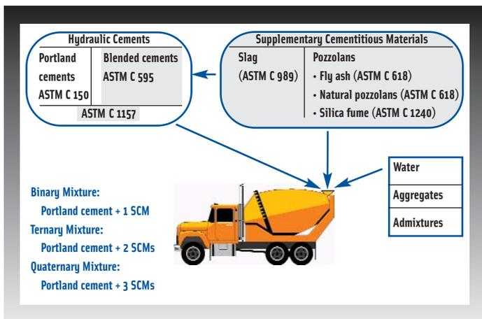
**Figure 1. Supplementary cementitious materials can be added directly to concrete, through use of a blended cement, or both.**
