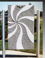
Panel 6: Plastic stencils and sandblasting created a swirl pattern. Stencils and sandblasting have recently been used for floors, too. (IMG14229)
