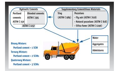
Figure 1. Supplementary cementitious materials can be added directly to concrete, through use of a blended cement, or both.
