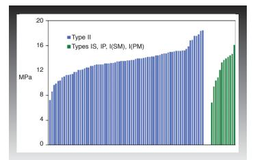
Figure 2. Generally, 1-day ASTM C 109 mortar strengths of ASTM C 595 cements are comparable to C 150 Type II cements. Later-age strengths follow this trend (Tennis 2001).
