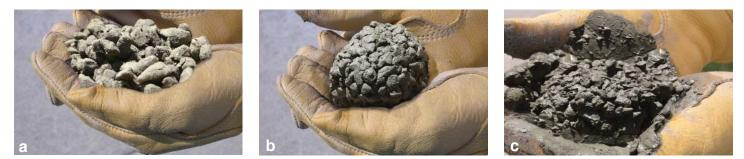
Figure 2. Samples of pervious concrete with different water contents formed into a ball: (a) too little water, (b) proper amount of water, (c) too much water. [IMG15595, IMG15596, IMG15597]
