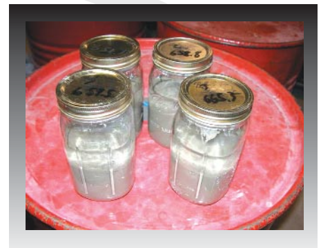
Fig. 1. In the mortar aggregate ratio test, a quality control method for mortar, samples are placed into jars of alcohol to stop cement hydration.
