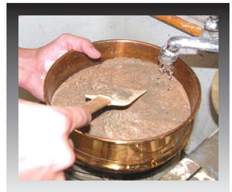
Fig. 2. Wet sieving over a number 100 sieve removes the fine mortar particles to determine how much aggregate is contained in the sample. Incidentally, a sand-only sample is also tested this way to provide a correction factor.
