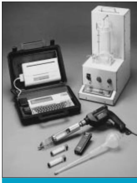
Figure 1. Equipment for the air-void analyzer. (67961)
