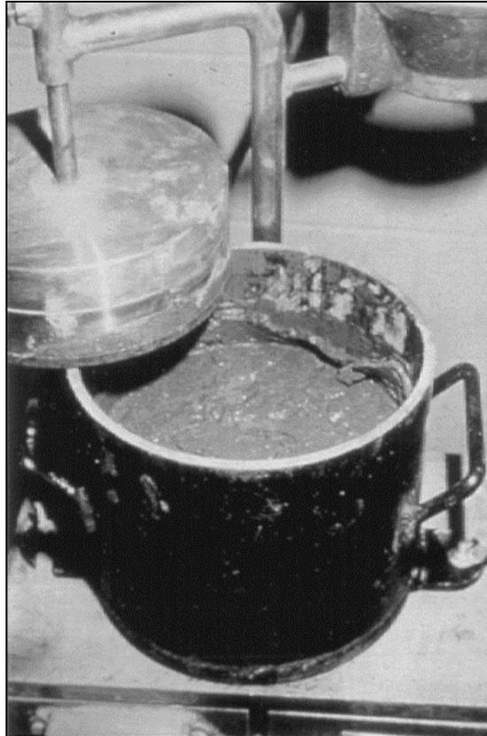
**Figure 4.1**—*Vebe consistency test with a ring of mortar on the consolidated sample.*
