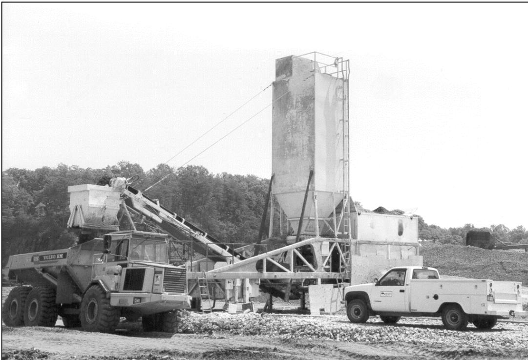
**Figure 4.8**—*Continuous-flow type plant producing RCC.*
