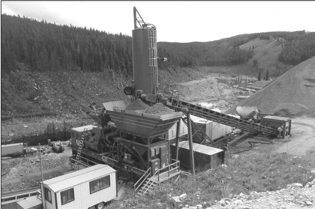
**Figure 4.7**—*Batch-type concrete plant producing RCC.*
