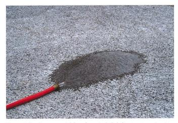
Figure 1. Pervious concrete's key characteristic is its open pore structure that allows high rates of water transmission. Trail in Athens Regional Park in Athens, TN, (A. Sparkman).
