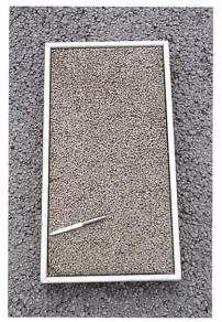
Figure 4. Pervious concrete is made with a narrow aggregate gradation, but different surface textures can be obtained through the use of different maximum sizes. The concrete in the box contained a 1/4-in. (6.5-mm) top size, while that below used a larger top size, 3/4 in. (20 mm) (J. Arroyo).
