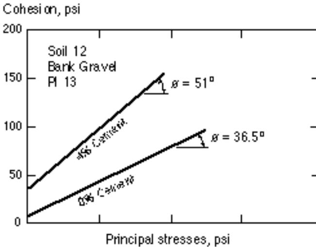
Fig. 8. Change in Triaxial Compressive Strength due to the Addition of Cement
