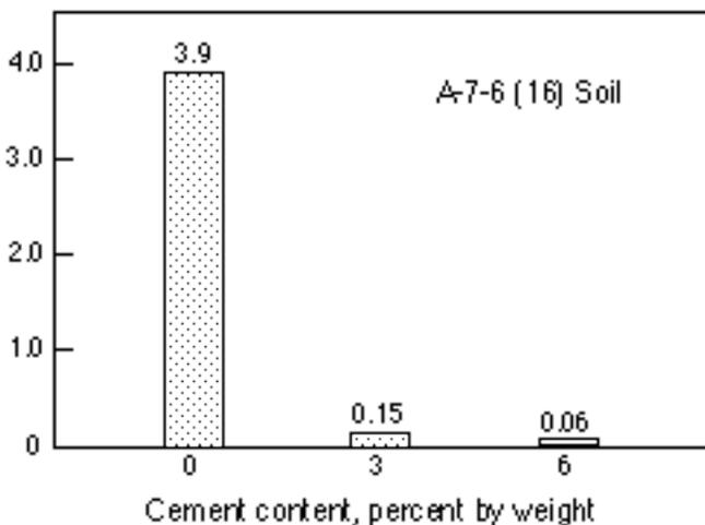
**Fig. 1. Effect of Cement on Swelling in the CBR Test**
