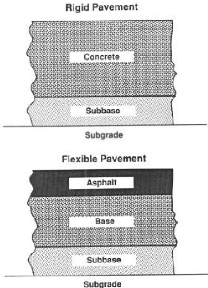
**Fig. 5. Terminology Used in Rigid and Flexible Pavement Layered Systems**
