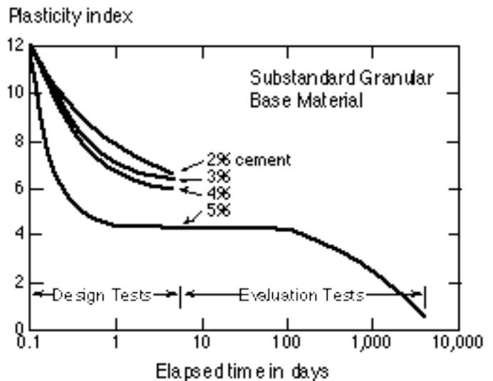
Fig. 6. Reduction in Plasticity Index Due to Cement Content and Time
