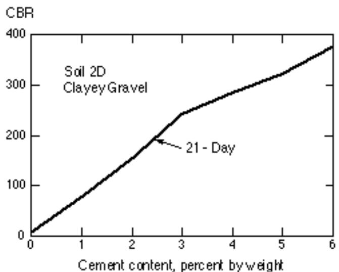
Fig. 7. California Bearing Ratio versus Cement Content
