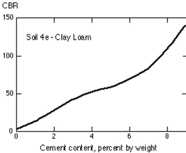
**Fig. 3. California Bearing Ratio versus Cement Content**
