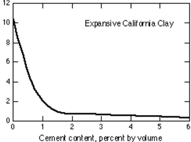
**Fig. 2. Expansion versus Cement Content, Highly Expansive Clay**
