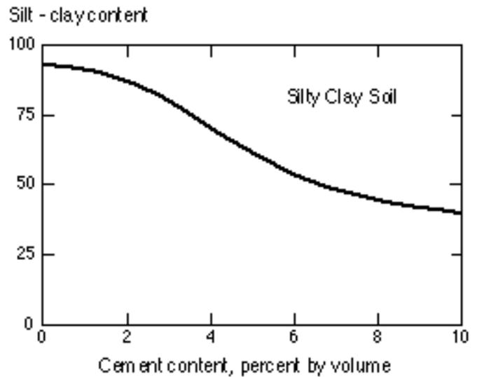
**Fig. 4. Reduction in Silt-Clay Content Due to Cement Modification**
