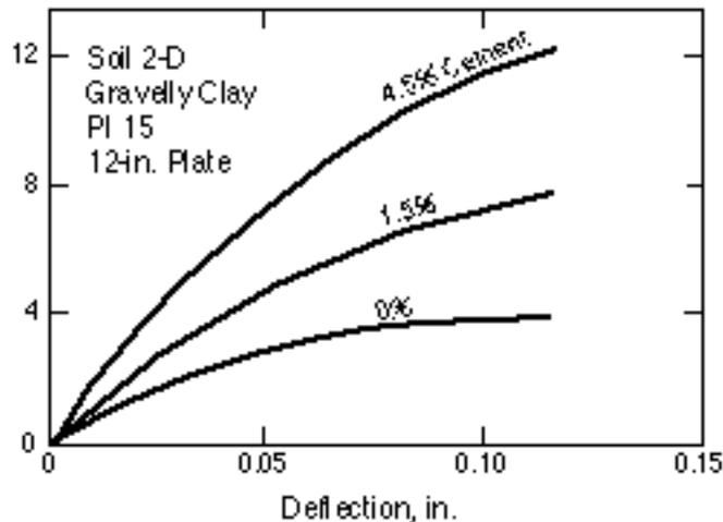
Fig. 9. Bearing Capacity versus Cement Content
