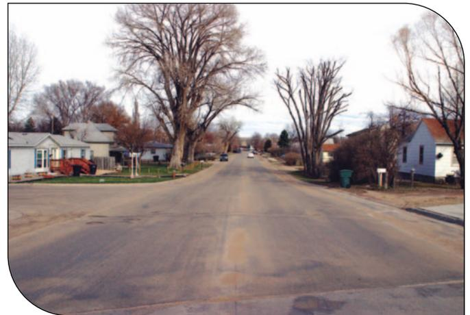
**Existing asphalt pavement on West 8th Street had deteriorated too much to accept a traditional ultra-thin whitetopping surface.**
