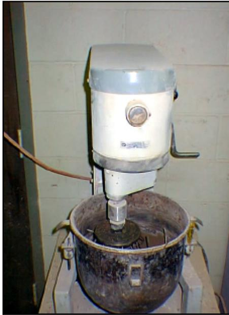
**Figure 23. Soil being mixed in laboratory mixer. (IMG15464)**
