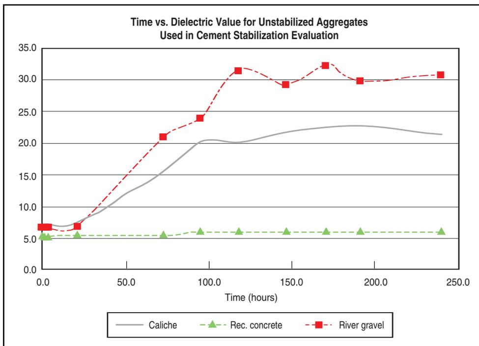
Figure 6. Results from TST on untreated materials.
