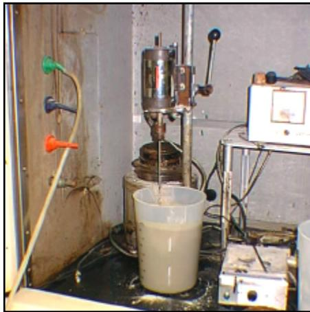
**Figure G1. Cement slurry being mixed in preparation for settling time test. (IMG15497)**
