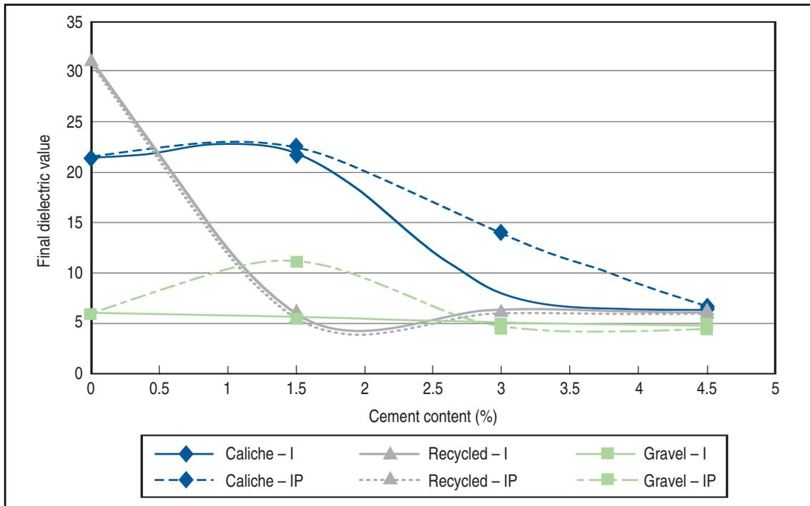
**Figure 8. Cement content vs. TST results.**
