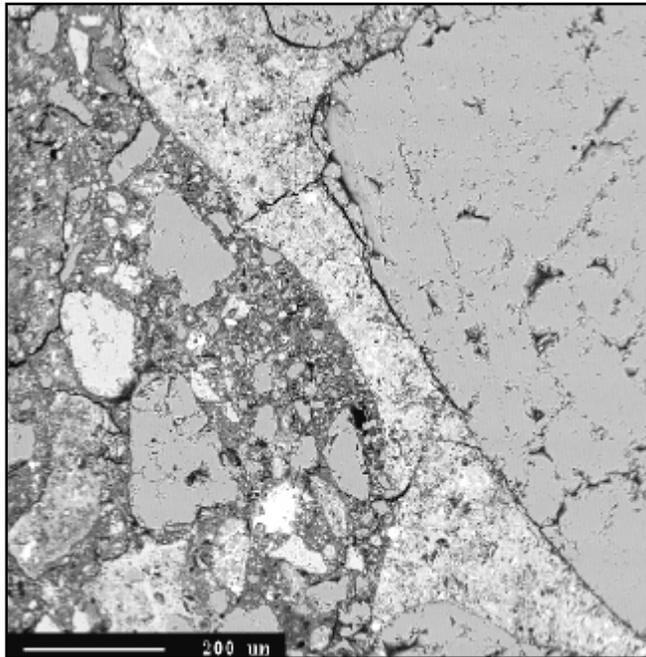
**Note the large quartz grain in the upper right of the image. The cement paste of the original concrete is seen as a lighter band surrounding this large aggregate. The new stabilizer (4.5% cement) is observed as a darker gray material on the left side of the image, 100x magnification.
