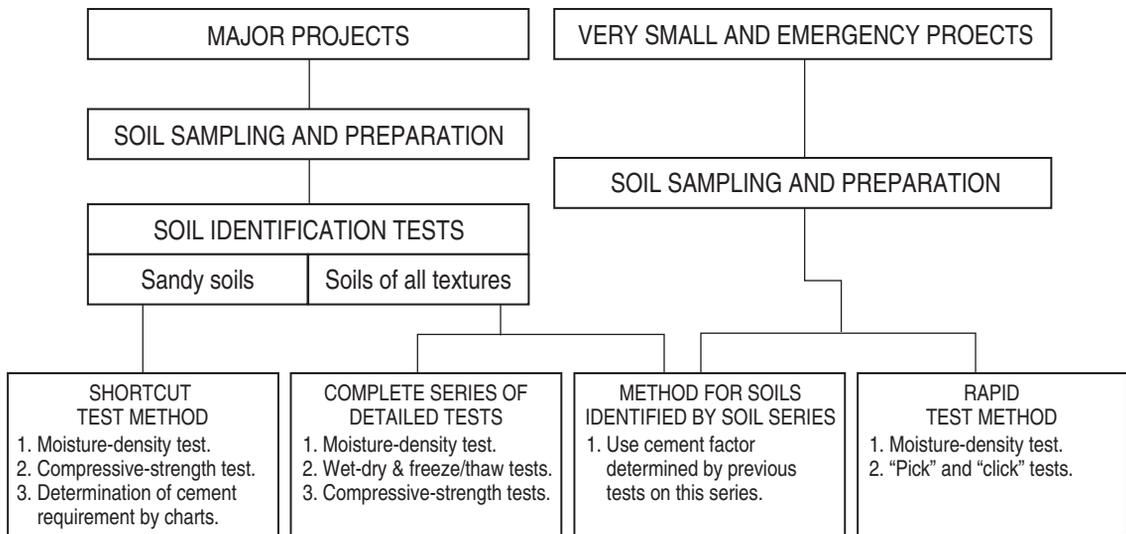
**Figure 2. Soil-cement laboratory testing methods (PCA, 1971).**
