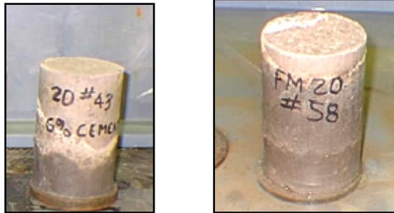
**Figure F2. Specimens After the Tube Suction Test stabilized with 5-minute old slurry (left) vs. four-hour old slurry (right). (IMG15496)**
