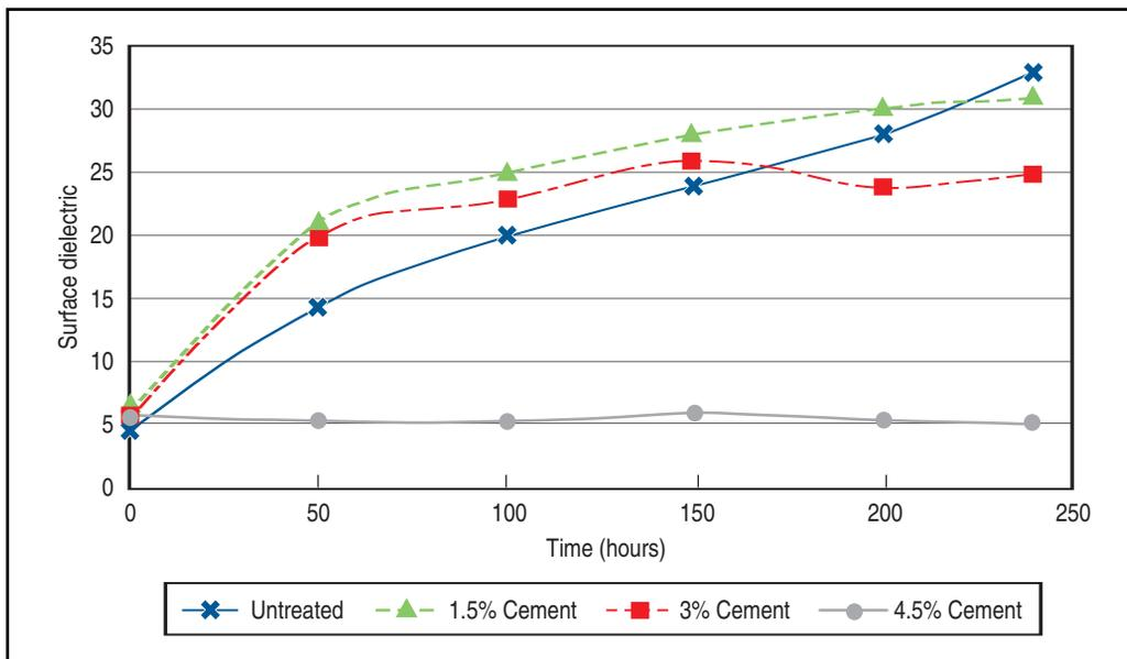
**Figure D8. Tube Suction Test on Houston recycled concrete (4 x 4.5 in.).**
