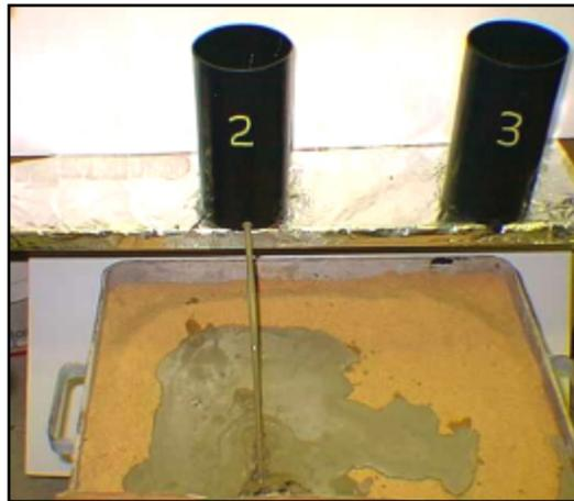
**Figure G2. Setup for the cement slurry settling time falling head flow-meter. (IMG15498)**
