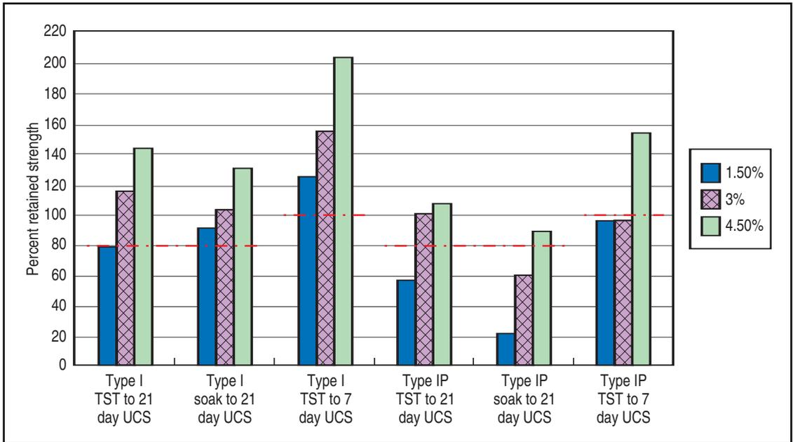
**Figure 15. Retained strength results for caliche.**
