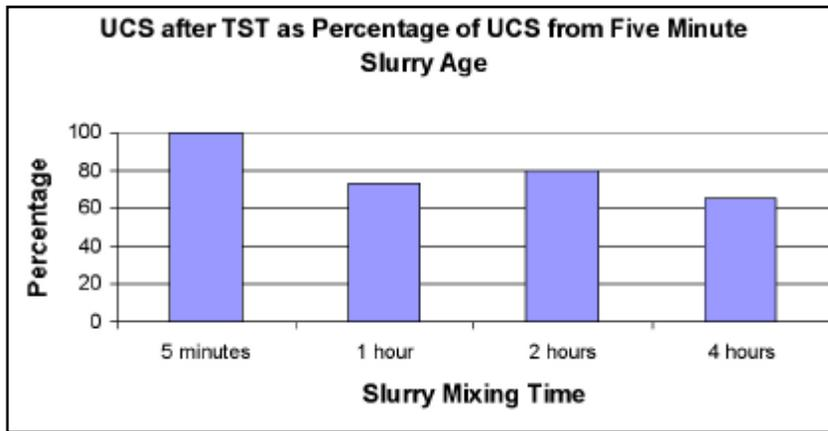
**Figure F4. Strengths after the Tube Suction Test as a percentage of strength from the five-minute-old slurry.**
