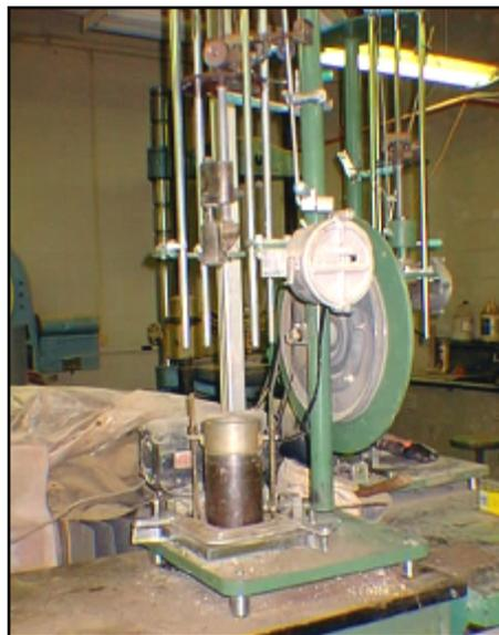
**Figure 24. Standard proctor for compaction of 4x6 test specimens. (IMG15477)**
