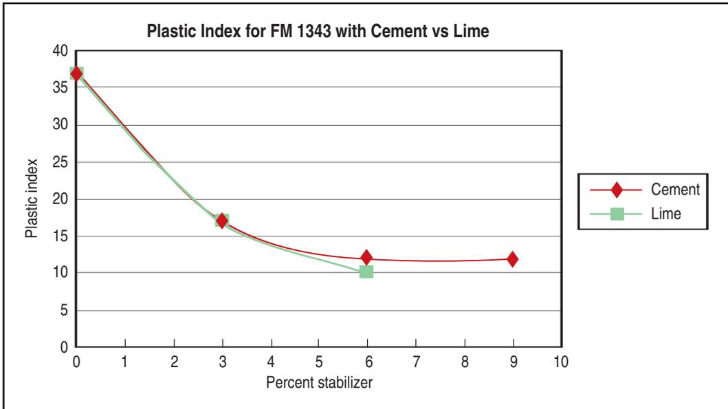
**Figure 20. Plastic index of soils after being stabilized.**
