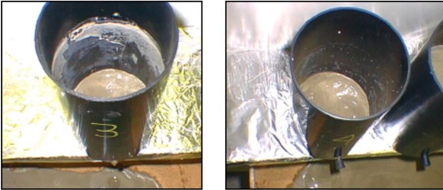
**Figure G4. Sludge remaining in test Cells from 30-minute (left) and 1-hour (right) slurry settling time tests. (IMG15500)**
