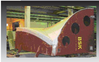
Figure 2 (above). Half-canopy in steel form.
