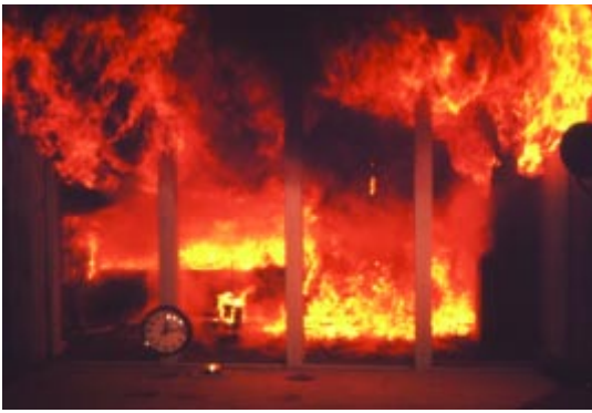
Fig. 18. When exposed to fire or unusually high temperatures, concrete can lose strength and stiffness. (55707)
