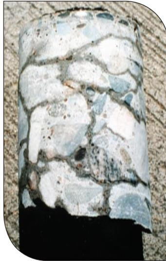
**Figure 6. Cracks can be more easily seen when the concrete has been wetted and is starting to dry. (Stark 1991a). (IMG12986)**
