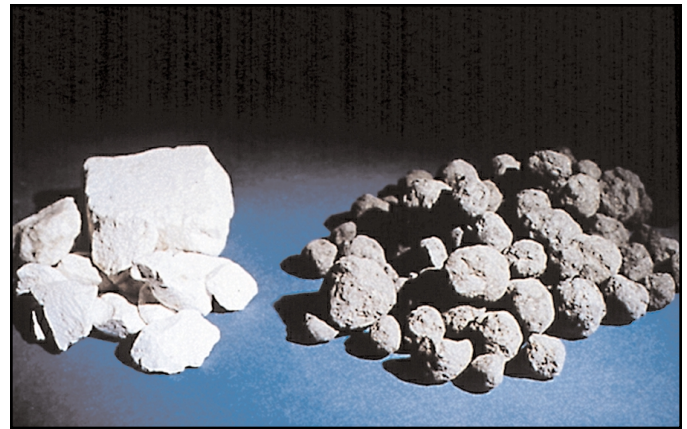
Fig. 1. Portland cements are manufactured by a process that combines sources of lime (such as limestone), silica and alumina (such as clay), and iron oxide (such as iron ore). Appropriately proportioned mixtures of these raw materials are finely ground and then heated in a rotary kiln at high temperatures, about 1450 °C (2640 °F), to form cement compounds. The product of this process is called clinker (nodules at right in above photo). After cooling, the clinker is interground with about 5% of one or more of the forms of calcium sulfate (gypsum shown at left in photo) to form portland cement. The calcium sulfate controls setting time, strength development, and drying shrinkage potential.
