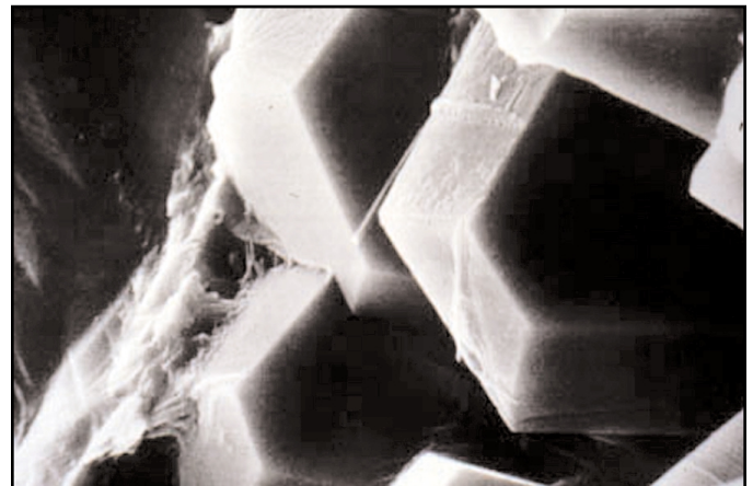
Fig. A-4 Scanning electron microscope micrograph of alite ( \text{C}_3\text{S} ) crystals. Magnification 3000X.
