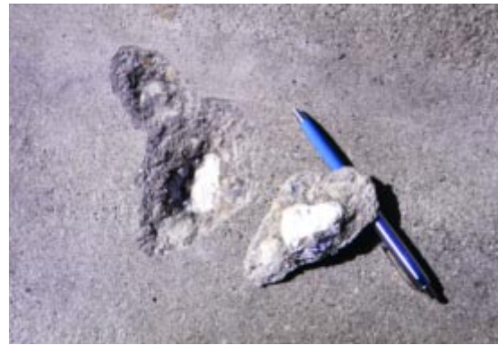
Fig. 8. Some aggregates absorb water and, upon freezing, expand to produce a popout. (0113)
