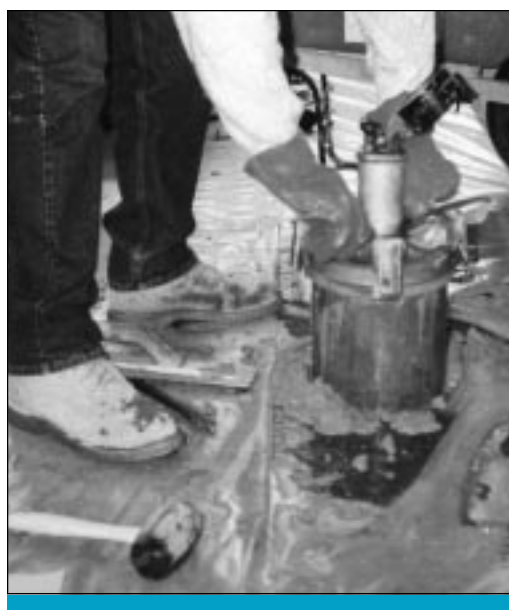
Figure 3. A Type B pressure meter used to measure total air content of fresh concrete. (P66113)
