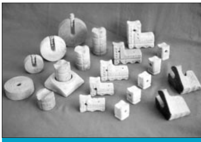
Figure 1. Bar supports and side-wall spacers made from high performance concrete featuring high strength (minimum 75 MPa (10,900 psi)); low permeability to air, water, and chloride ions; high resistance to chemicals; and geometrically and materially designed to become an integral part of the host concrete structure. (67925)
