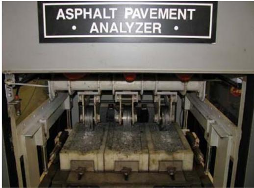
(a) Asphalt Pavement Analyzer (APA)
