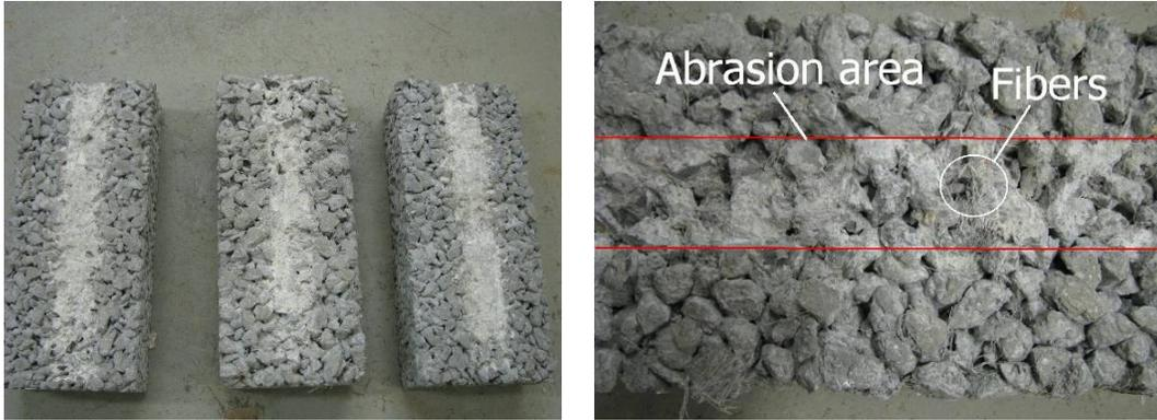
Figure 4 Specimens after loaded wheel abrasion test
