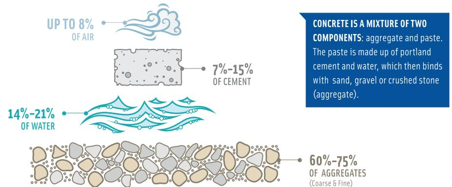
**CONCRETE IS A MIXTURE OF TWO COMPONENTS:** aggregate and paste. The paste is made up of portland cement and water, which then binds with sand, gravel or crushed stone (aggregate).
