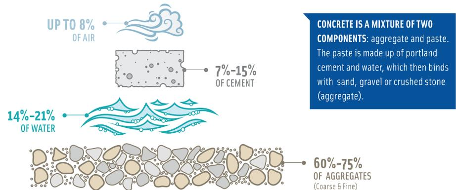
**CONCRETE IS A MIXTURE OF TWO COMPONENTS:** aggregate and paste. The paste is made up of portland cement and water, which then binds with sand, gravel or crushed stone (aggregate).
