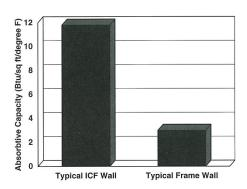
The heavy concrete of the ICF wall gives it the heat-absorbing property of "thermal mass". This smooths out swings in temperature over time. So the house does not tend to overheat or get suddenly chilly as the furnace or air conditioner cycles on and off.
