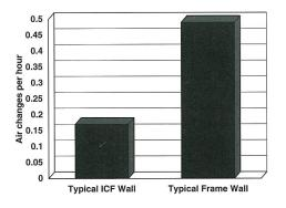
The interlocking foam faces, sealed with continuous concrete in the center, make ICF walls exceptionally airtight. So drafts are cut sharply. In tests, houses built of ICFs had only about one-third to one-half as much air infiltration as the typical frame house.
