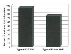
The continuous layer of foam insulation along the ICF wall helps keep the temperature the same everywhere. It virtually eliminates the "cold spots" that can occur in frame walls along the studs or at gaps in the insulation.
