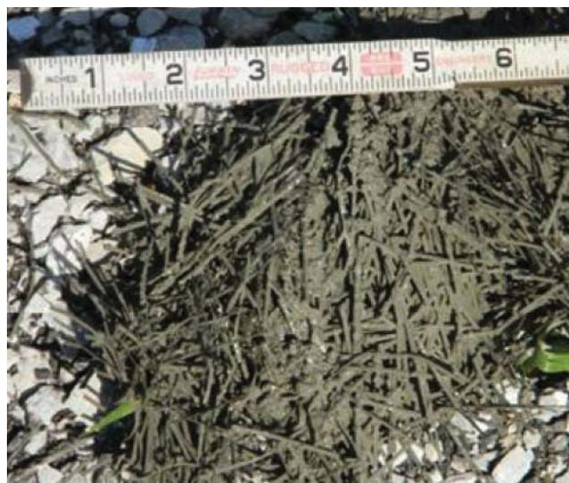
Figure 2-3. Synthetic fibers
