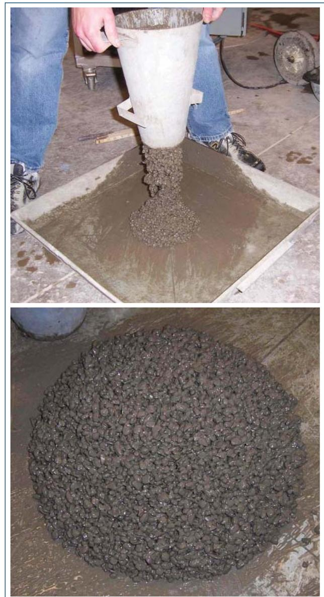
**Figure 3-6. Fresh pervious concrete**
