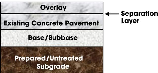
Figure 2-4. Typical cross-section of unbonded overlay over concrete
