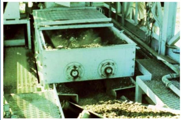
Figure 5-12. Mobile RCC pugmill mixing plant and mixing chamber
