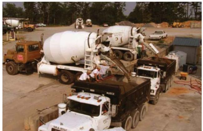
Figure 5-11 Ready-mix transit trucks dumping into haul trucks
