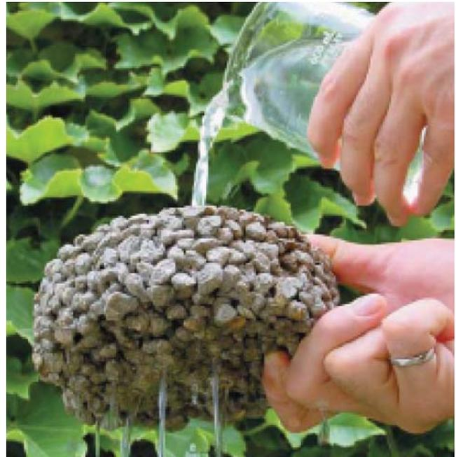
Figure 3-4. Pervious concrete
