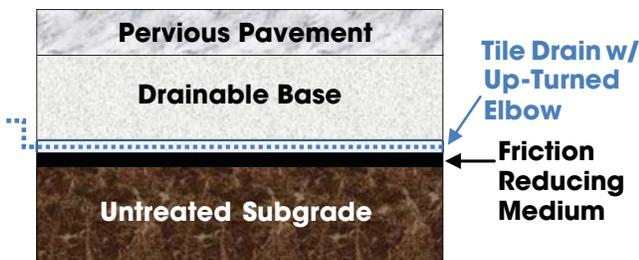
Figure 3-9. Schematic of pervious partial exfiltration pavement design
