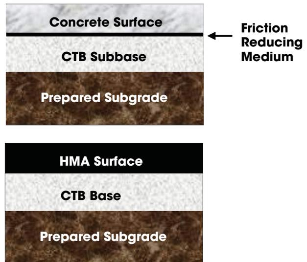
Figure 6-2. Typical pavement cross-sections showing CTB layers
