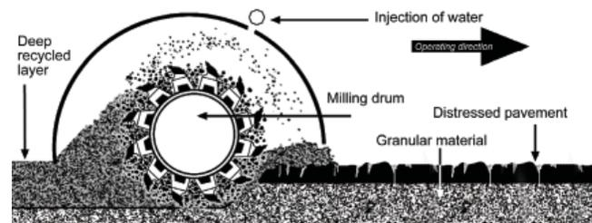
Figure 7-1. Schematic of the mixing chamber of a reclaimer machine
