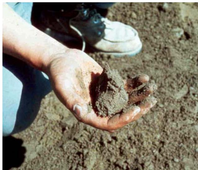
Figure 5-6. RCC material looks drier than conventional concrete
