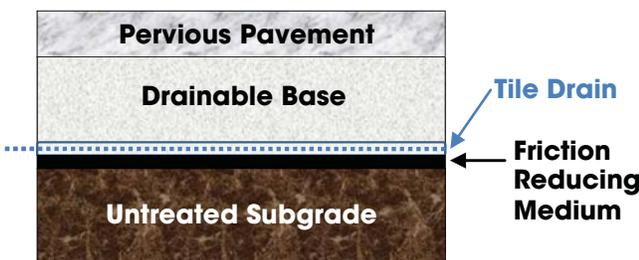
Figure 3-10. Schematic of pervious no exfiltration pavement design
