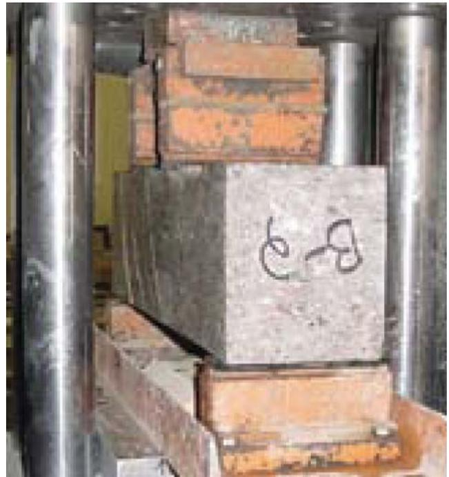
Figure 5-7. Flexural beam testing
