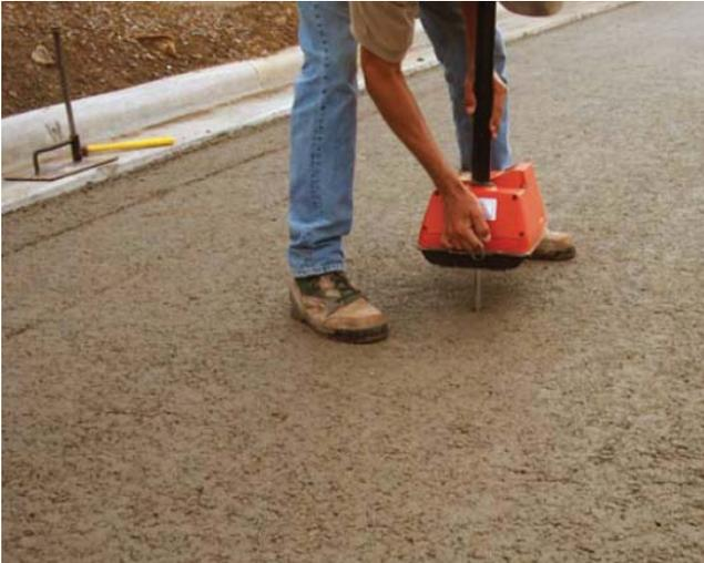
Figure 5-15. RCC in-place density measurement
