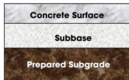
Figure 1-1. Schematic of typical concrete pavement cross-section
