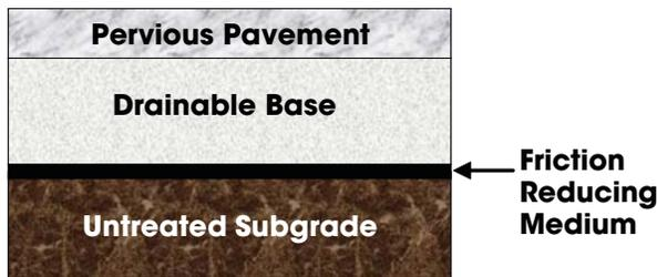
Figure 3-8. Schematic of pervious full exfiltration pavement design
