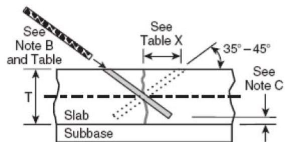
Figure 10-3. Cross-section of concrete pavement showing stitching
