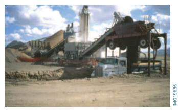
Figure 6-3. Central plant pugmill mixer with bottom dump trailer used for storage hopper at Santa Cruz River, Arizona.
