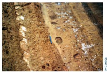
Figure 3-1. "Swiss cheese" appearance of soil-cement with clay balls.
