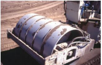
Figure 5-32. Ribbed drum used to create indentation in surface of soil-cement.
