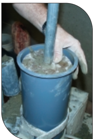
Figure 8. Preparation of RCC cylinder using the Vebe Table.
