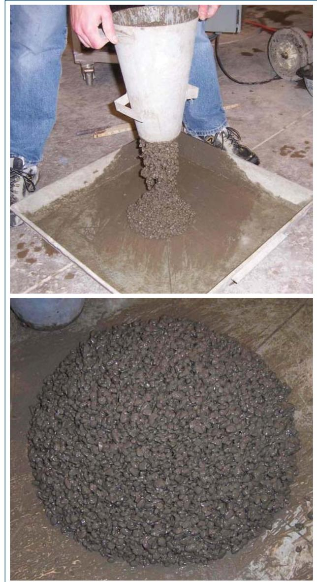
**Figure 3-6. Fresh pervious concrete**
