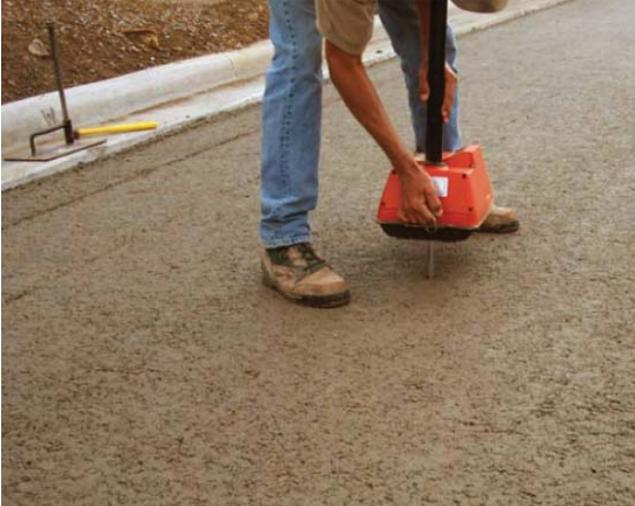
Figure 5-15. RCC in-place density measurement
