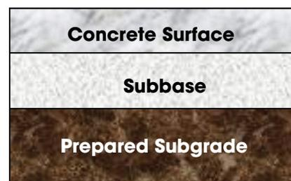
Figure 1-1. Schematic of typical concrete pavement cross-section
