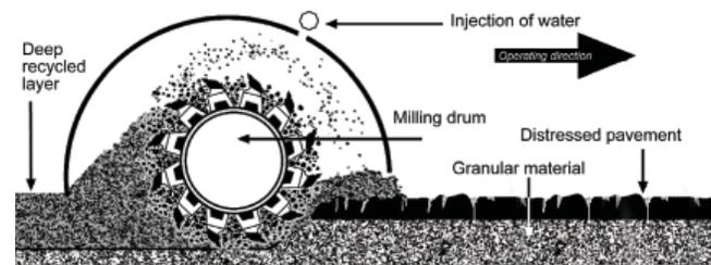
Figure 7-1. Schematic of the mixing chamber of a reclaimer machine
