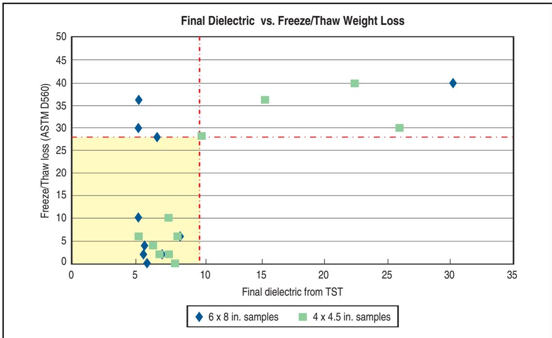
**Figure D10. TST results with freeze/thaw durability test results.**
