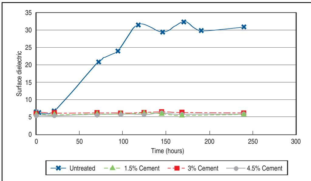
**Figure D7. Tube Suction Test on Houston recycled concrete (6 x 8 in.).**
