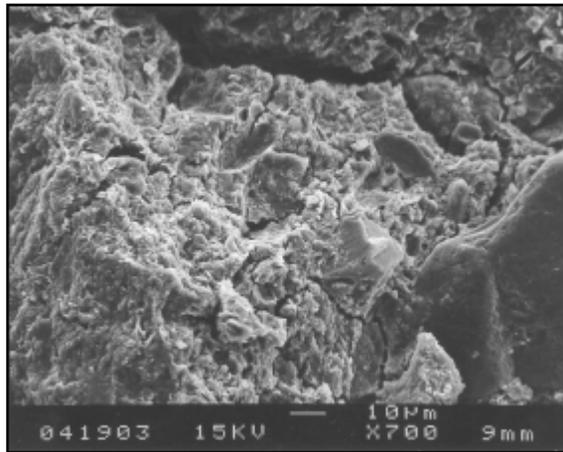
**Figure E2. FM 1343 pulverized with 3% cement. (IMG15494)**
