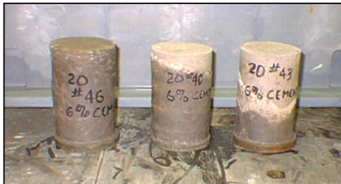
**From left to right: dry application to dry soil, dry application to moist soil, and slurry application to moist soil**
