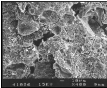
Figure A2. Pharr caliche with 3.0% cement. (IMG15489)
