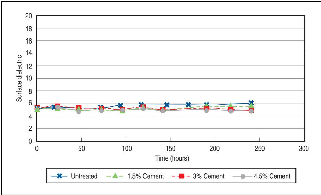
**Figure D5. Tube Suction Test on Yoakum river gravel (6 x 8 in.).**
