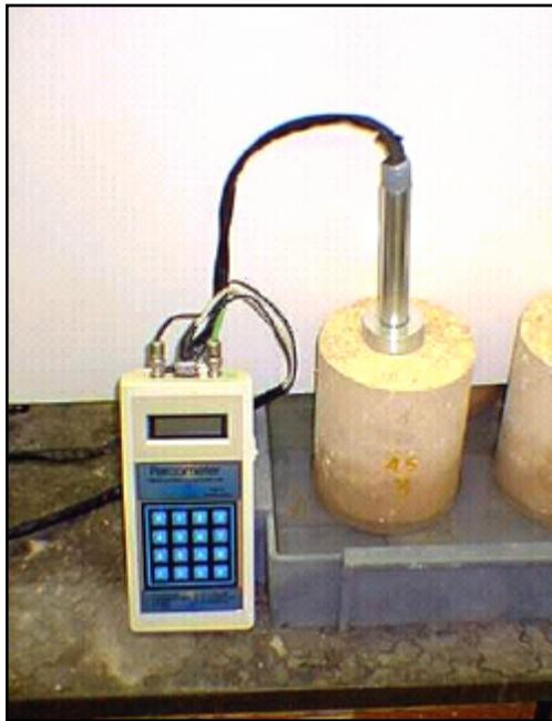
**Figure B3. Base specimens in the TST. (IMG15507)**
