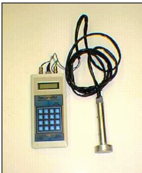
**Figure B1. Adek Percometer. (IMG15505)**
