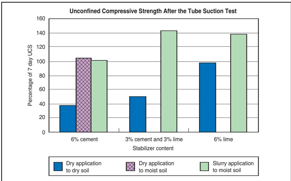
**Figure 37. Moisture susceptibility results comparing the strength After capillary rise to the 7-day strength.**
