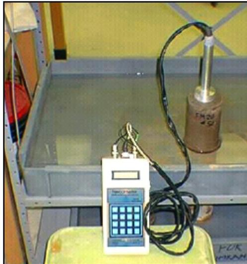
**Figure B2. Setup of the TST for subgrade soils. (IMG15506)**
