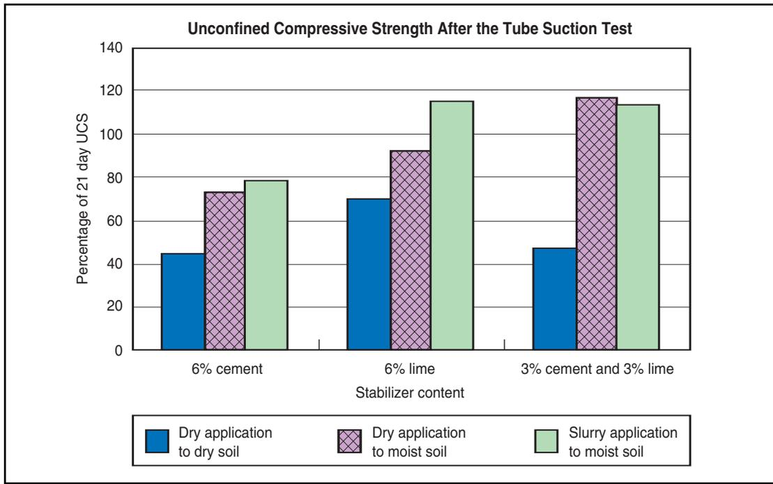
**Figure 35. UCS after the Tube Suction Test as a percentage of their 21-day curing strength.**
