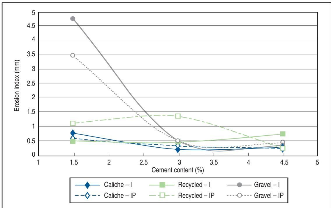
**Figure 11. Cement content vs. erosion index.**
