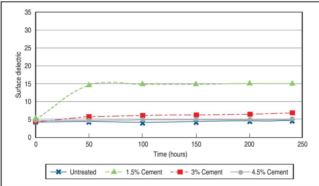
**Figure D6. Tube Suction Test on Yoakum river gravel (4 x 4.5 in.).**
