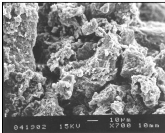
**Figure E1. FM 1343 pulverized with 3% lime. (IMG15493)**
