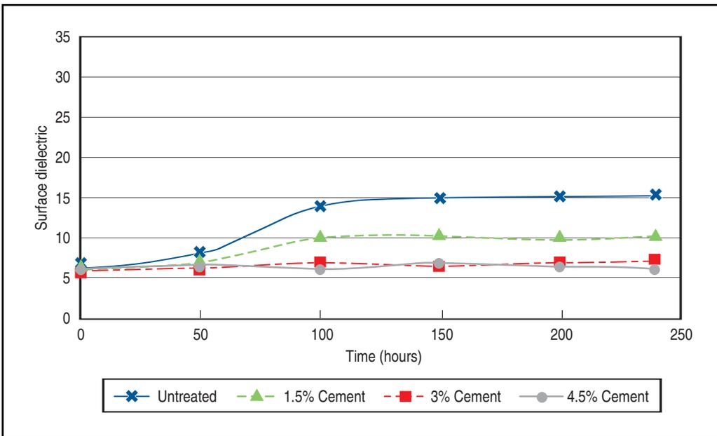
**Figure D2. Tube Suction Test on crushed limestone (4 x 4.5 in.).**
