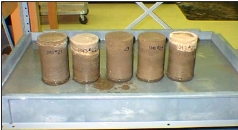
**From left to right: 3% cement, 6% cement, 3% lime, 6% lime, 3% cement and 3% lime
