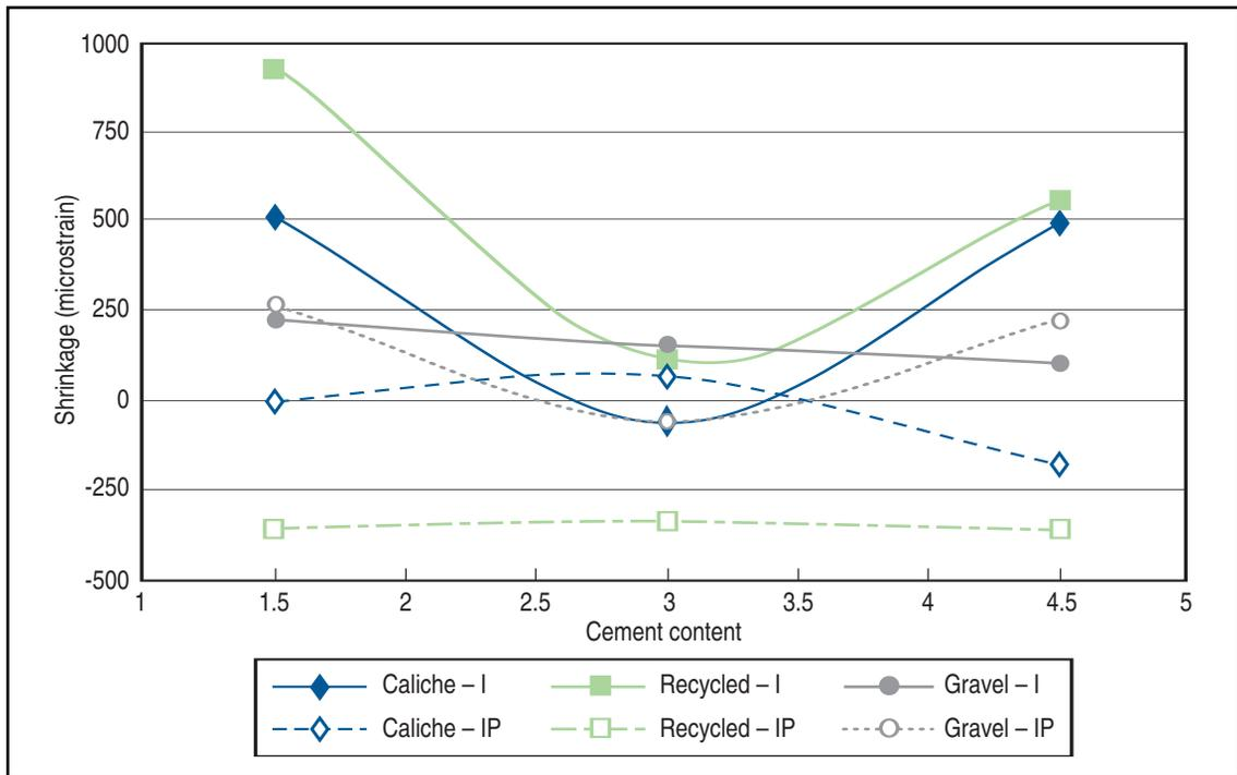
**Figure 10. Cement content vs shrinkage.**
