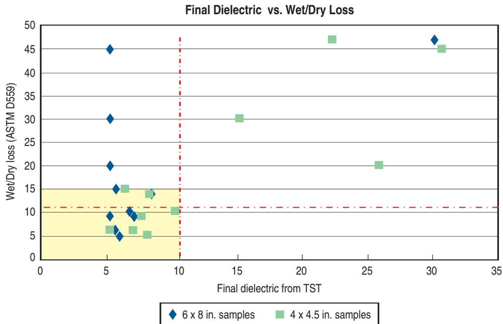
**Figure D9. TST results with wet/dry durability test results.**
