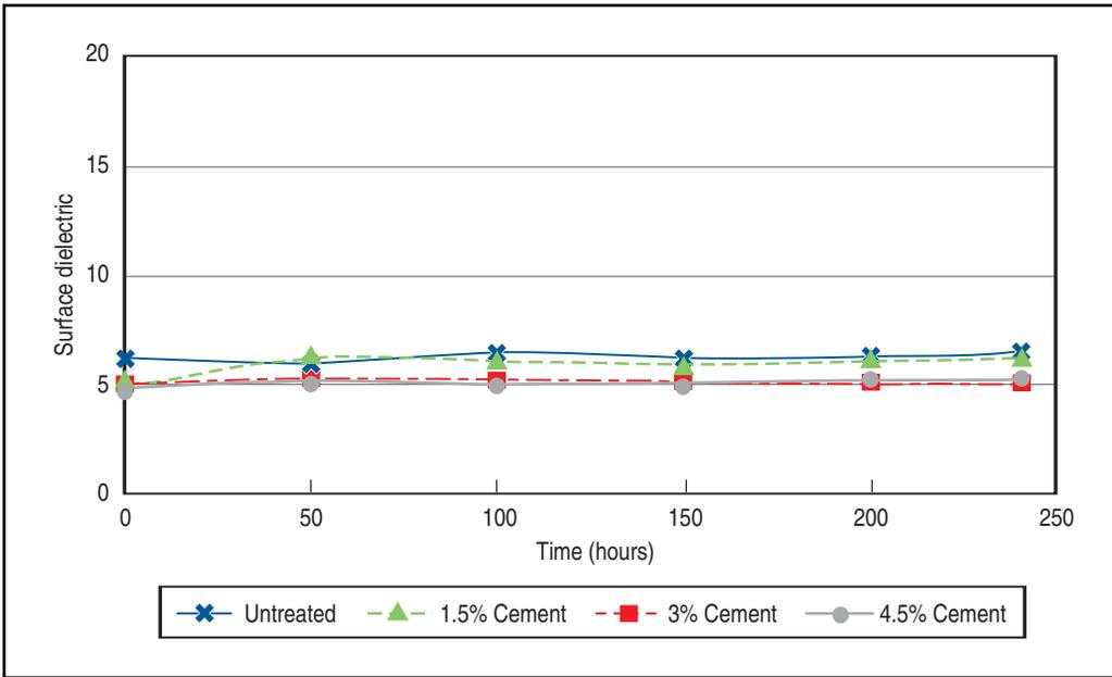
**Figure D1. Tube Suction Test on crushed limestone (6 x 8 in.).**
