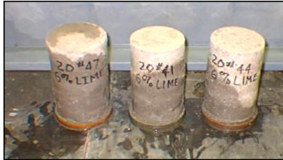
**From left to right: dry application to dry soil, dry application to moist soil, and slurry application to moist soil**
