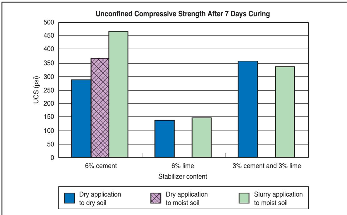
**Figure 36. Results from 7-day strength testing.**
