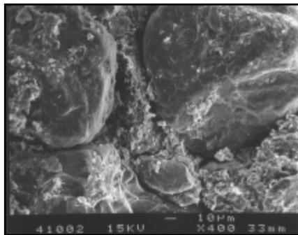
**Figure A1. Pharr caliche with 1.5% cement. (IMG15488)**
