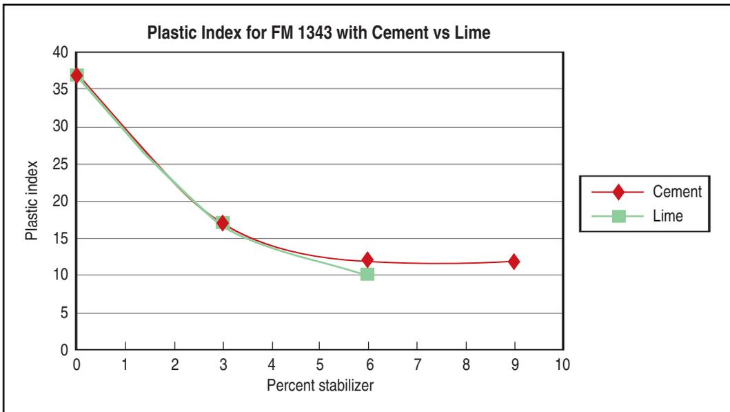
**Figure 20. Plastic index of soils after being stabilized.**
