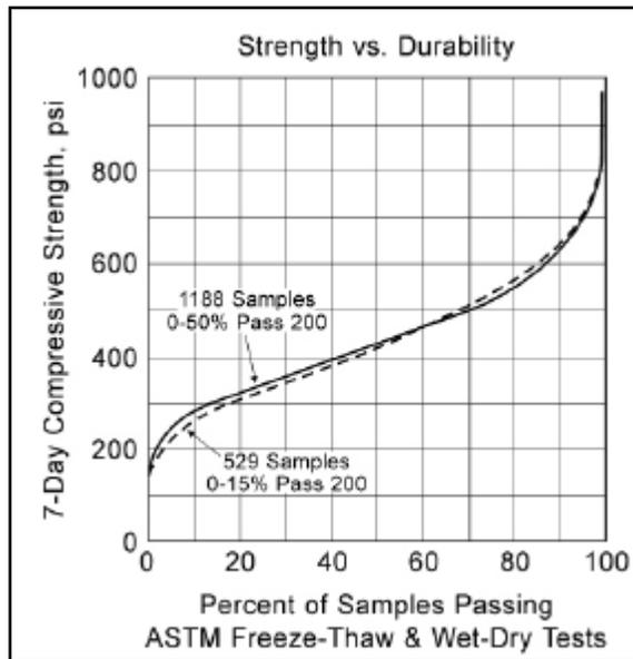
**Figure I. Relationship between strength and durability (PCA).**
