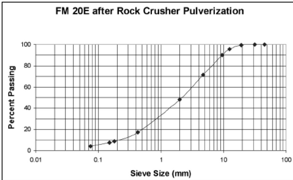
**Figure 22. Gradation curve for Level I pulverization.**
