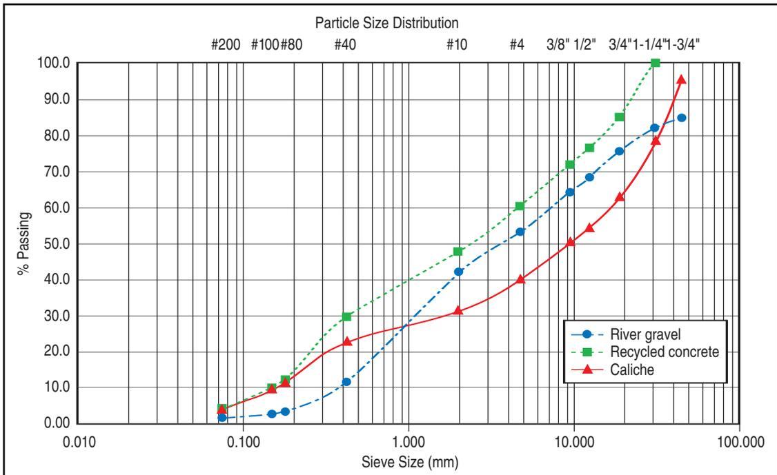
**Figure 5. Gradation of base materials.**
