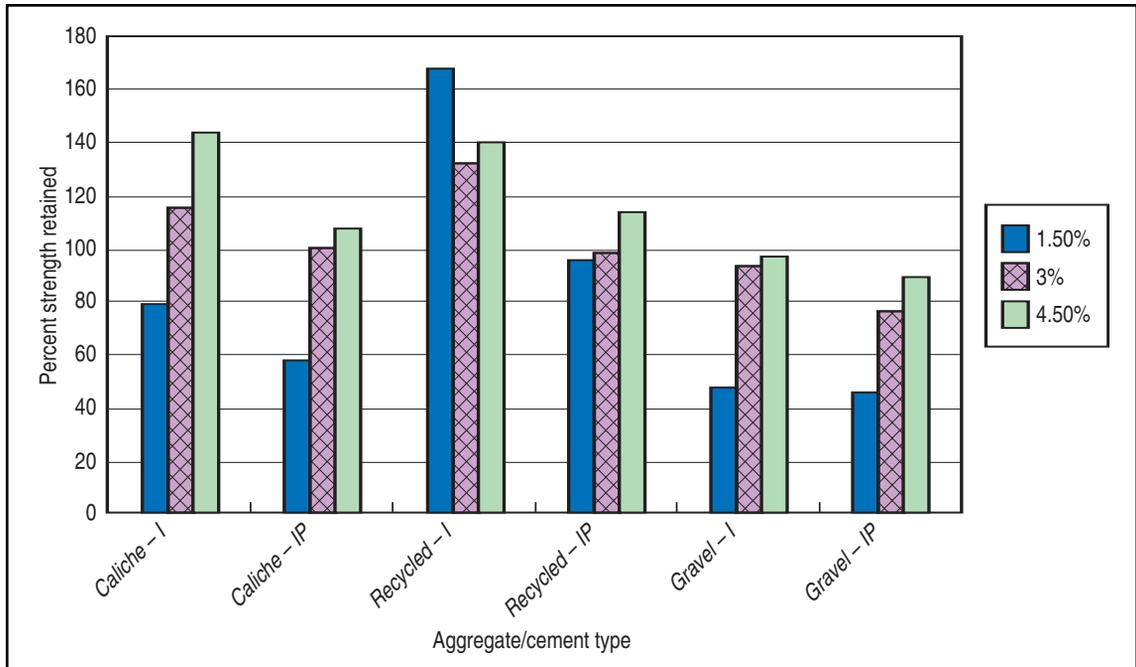
**Figure 9. Retained strength increases with increasing cement content.**
