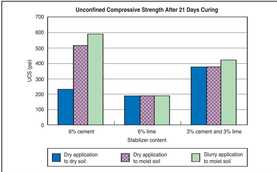
**Figure 29. UCS for FM 20 soil after 21 days curing time.**
