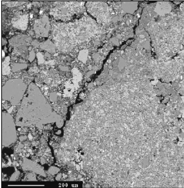
Note the heterogeneous nature of the aggregates and cement paste.
