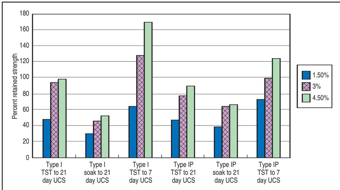
**Figure 17. Retained strength results for gravel.**
