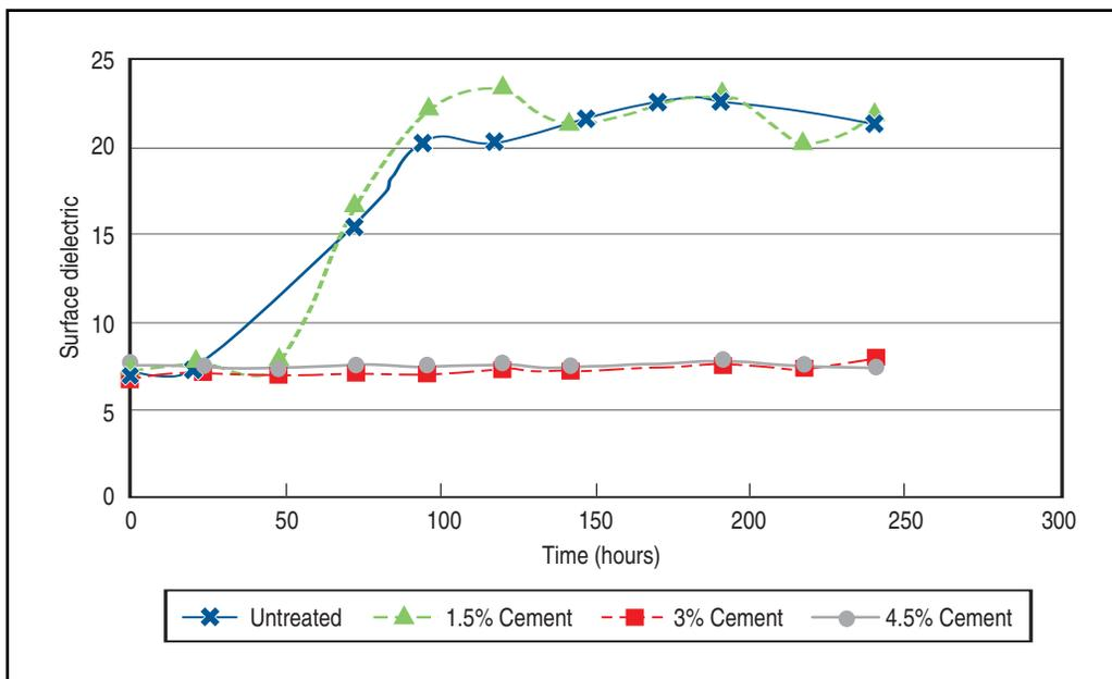
**Figure D3. Tube Suction Test on Pharr caliche (6 x 8 in.).**
