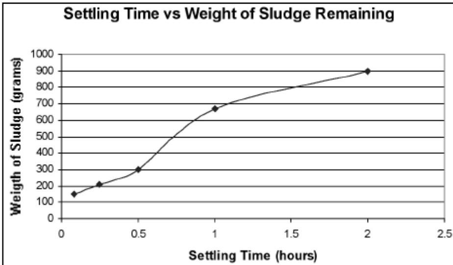
**Figure G5. Weight of sludge remaining at the end of the cement slurry settling time falling head flow-meter testing.**
