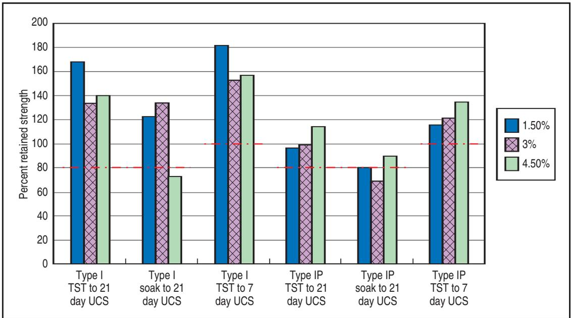
**Figure 16. Retained strength results for recycled aggregate.**
