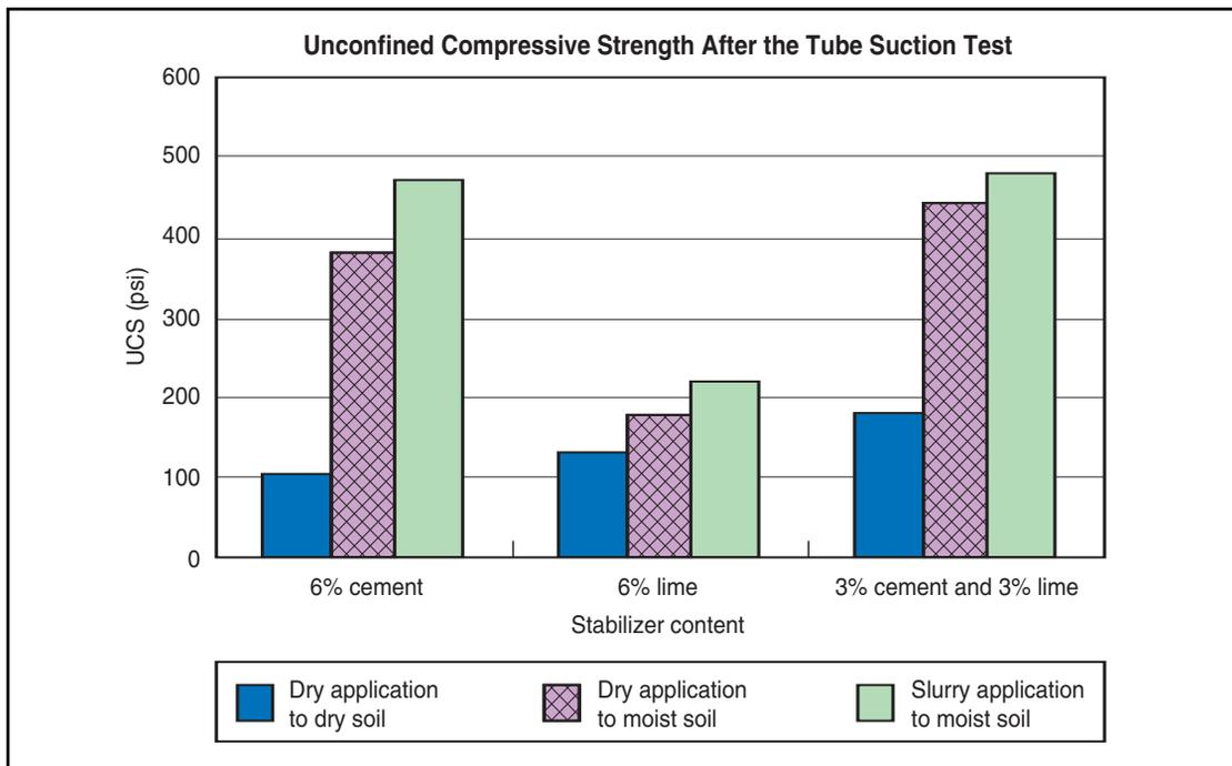
**Figure 34. UCS for FM 20 after the Tube Suction Test.**
