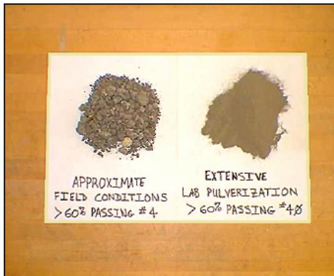
Figure 21. Pulverization levels used in study. (IMG15467)
