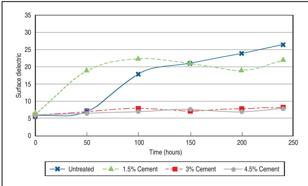
**Figure D4. Tube Suction Test on Pharr caliche (4 x 4.5 in.).**
