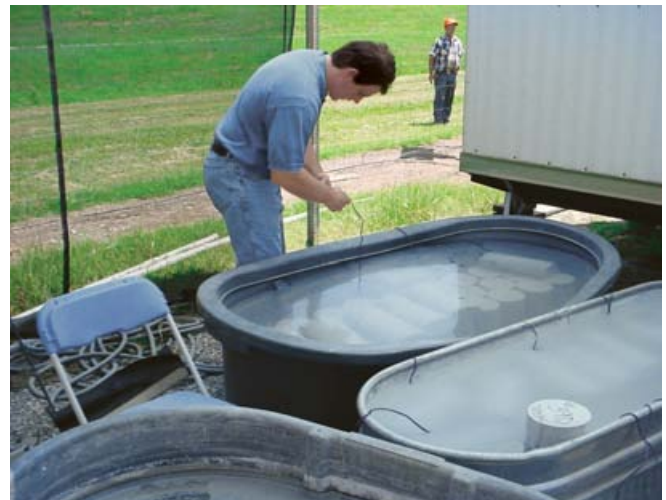
Figure 22. Measuring concrete temperatures to develop a maturity curve. (Courtesy of Mike Fox, Engius.)
