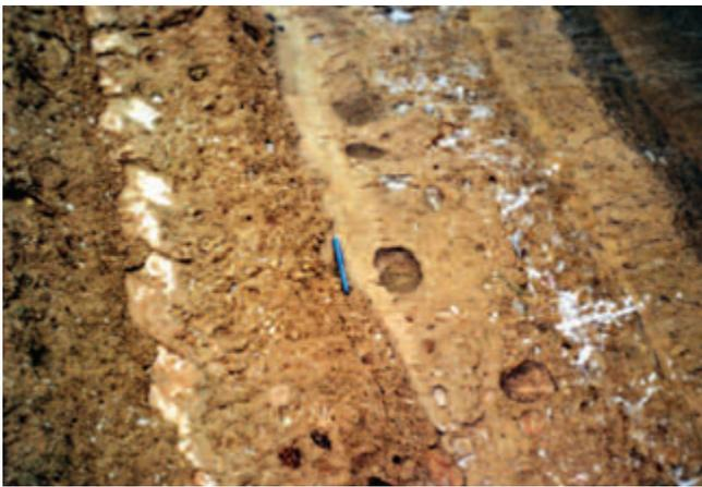
Figure 3-1. “Swiss cheese” appearance of soil-cement with clay balls.
