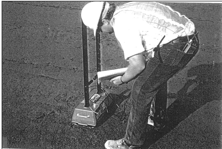
**Figure 5.4**—Double-probe nuclear density gauge.
