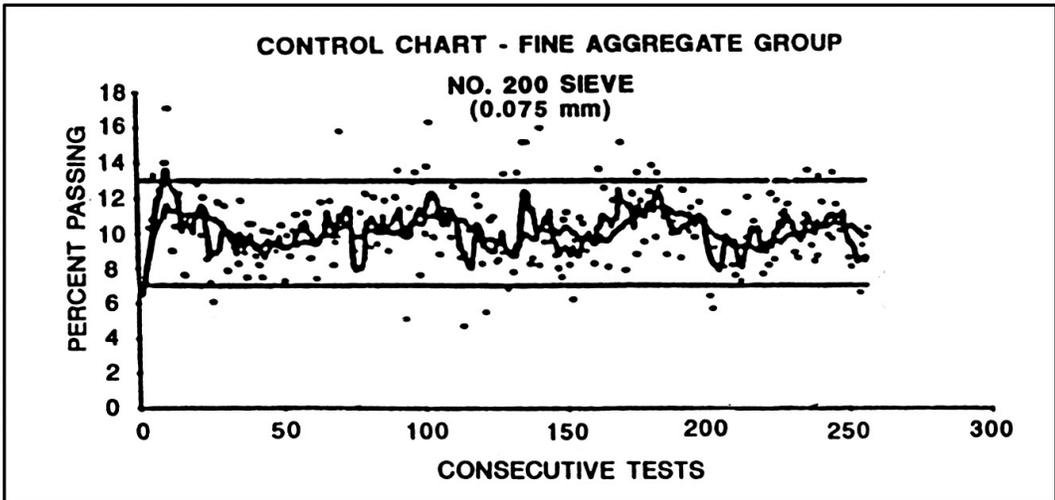
*Figure 4.4—Typical control charts for tracking fine aggregate grinding results by selected individual sieves.*
