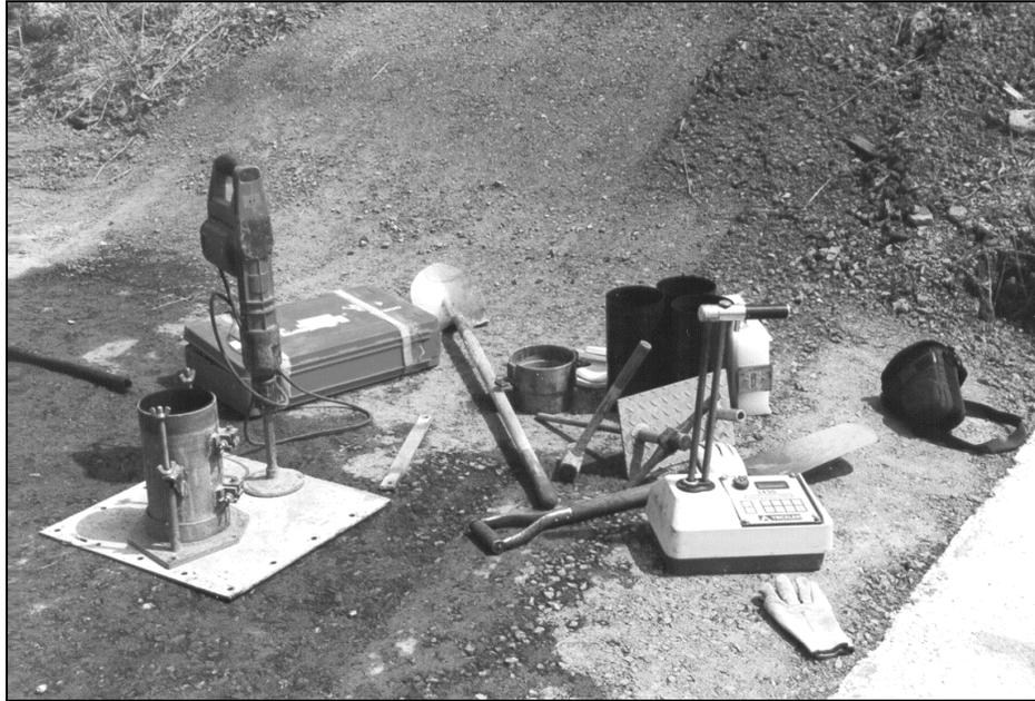
**Figure 5.3**—Vibrating hammer for preparation of RCC cylinders, and single-probe nuclear density gauge.
