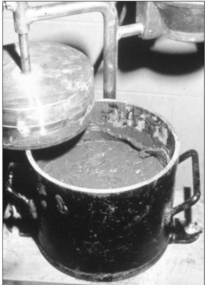
Figure 8.8. Ring of mortar formed between surcharge and inside of Vebe container
