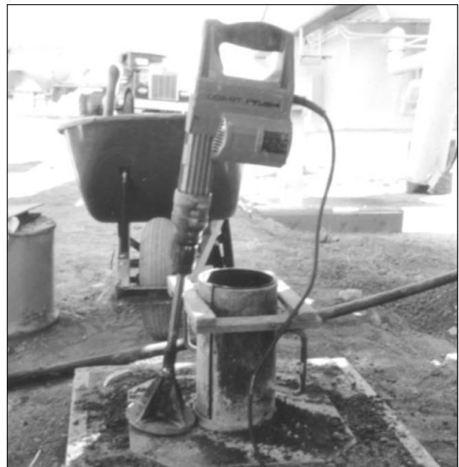
**Figure 8.3.** Modified Hilti hammer used to prepare RCC cylinder in the field
