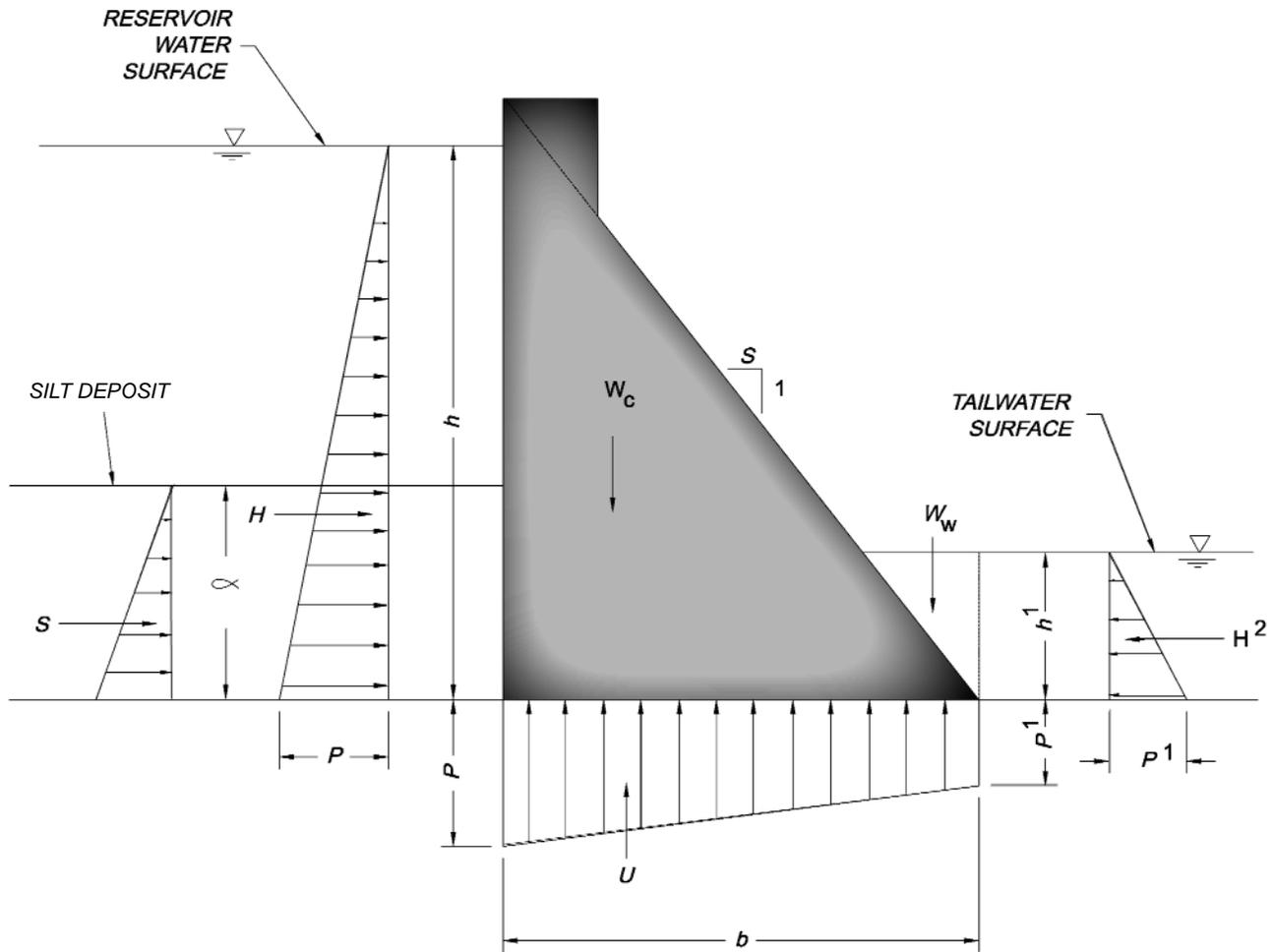
Figure 4.1. Loads on typical gravity section
