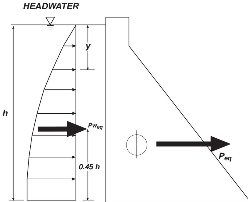
Figure 4.2. Seismically loaded gravity dam, non-overflow monolith
