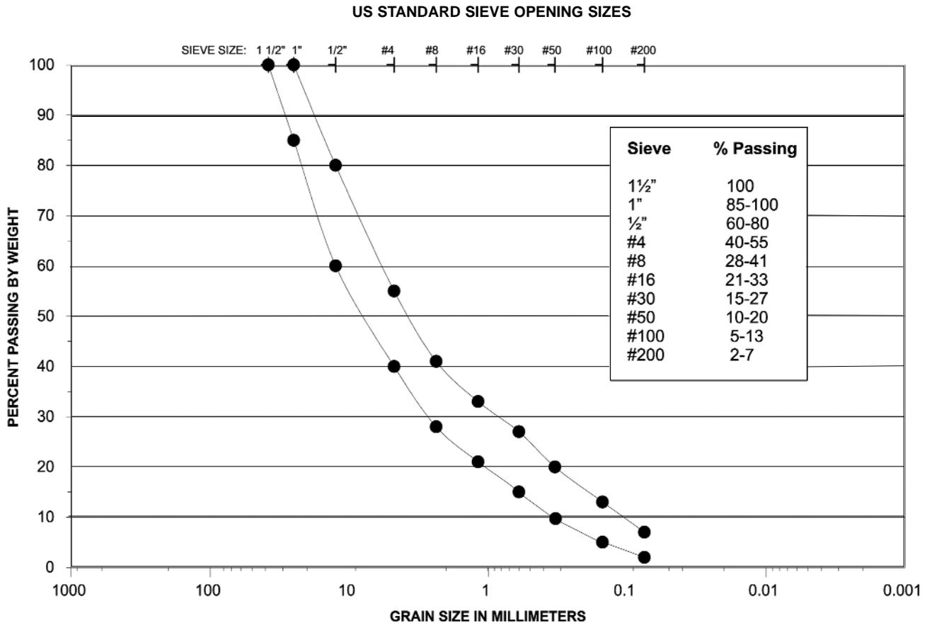
Figure 8.1. Typical aggregate gradation band for a small RCC dam
