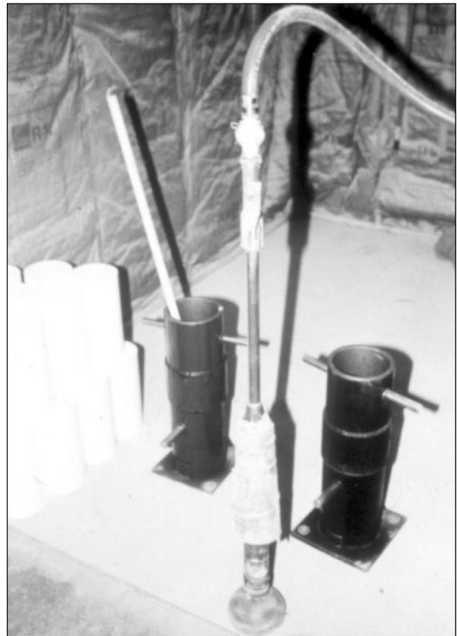
**Figure 8.5.** A pneumatic pole tamper used to make RCC cylinders
