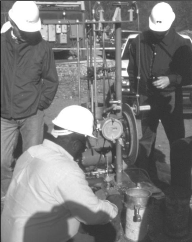
**Figure 8.2.** Modified Proctor compaction equipment being used to produce an RCC cylinder
