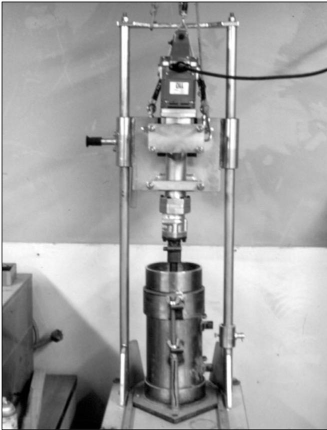
**Figure 8.4.** A mounted Kango hammer for use in preparing laboratory RCC cylinders
