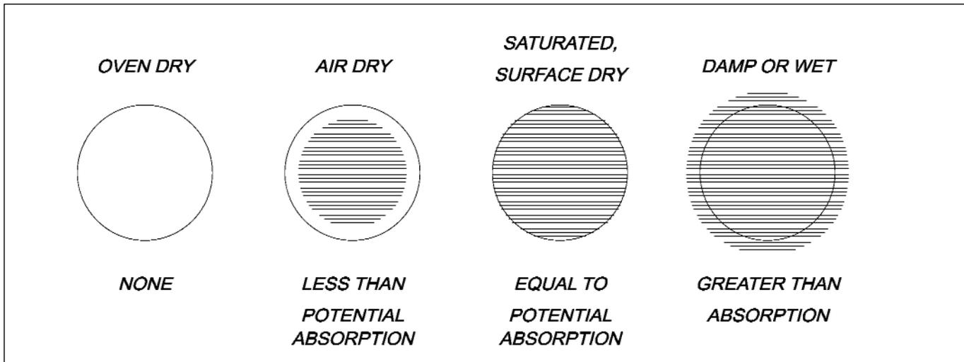
Figure 8.6 . Various moisture conditions of aggregate
