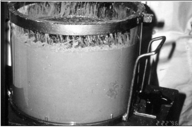
Figure 8.9. Clear plastic container being used to determine Vebe time
