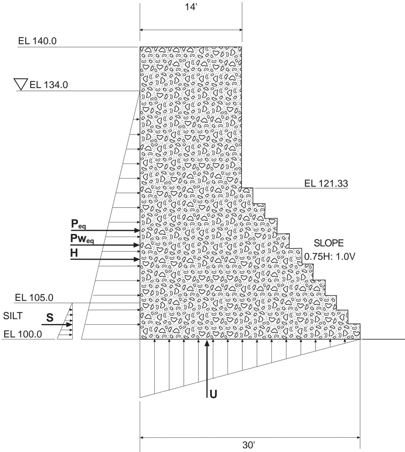
Figure A3. Loading Condition 3 Maximum Pool—Partial Section
