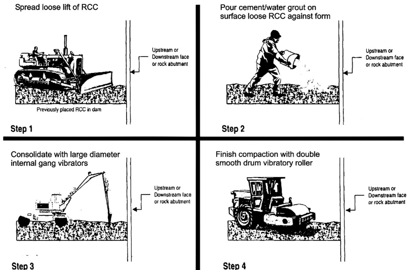
Figure 7.9 Grout Enriched RCC Method (Courtesy of William Moler)
