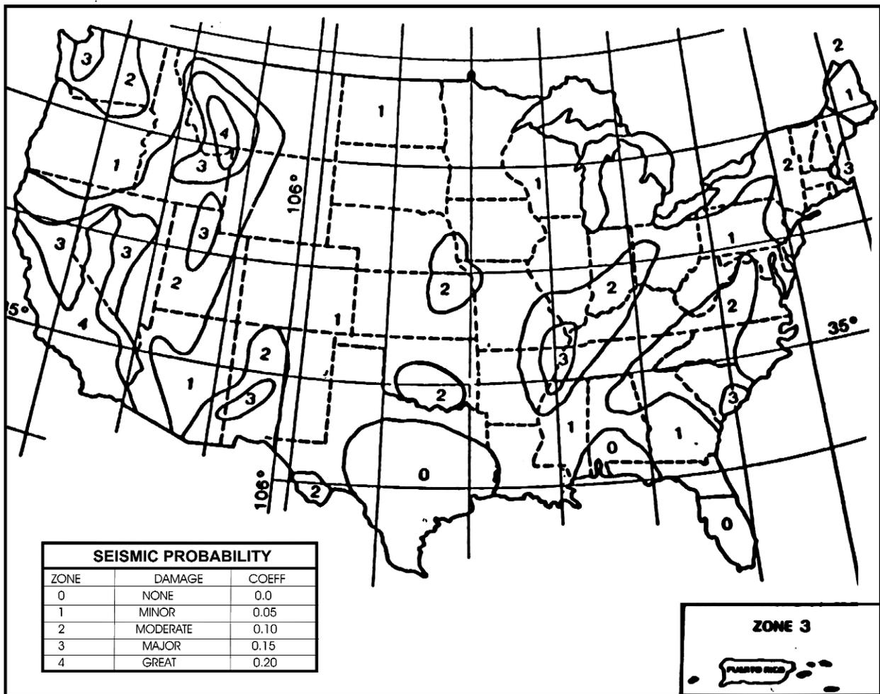
Figure 4.3. Seismic zone map of the contiguous United States and Puerto Rico
