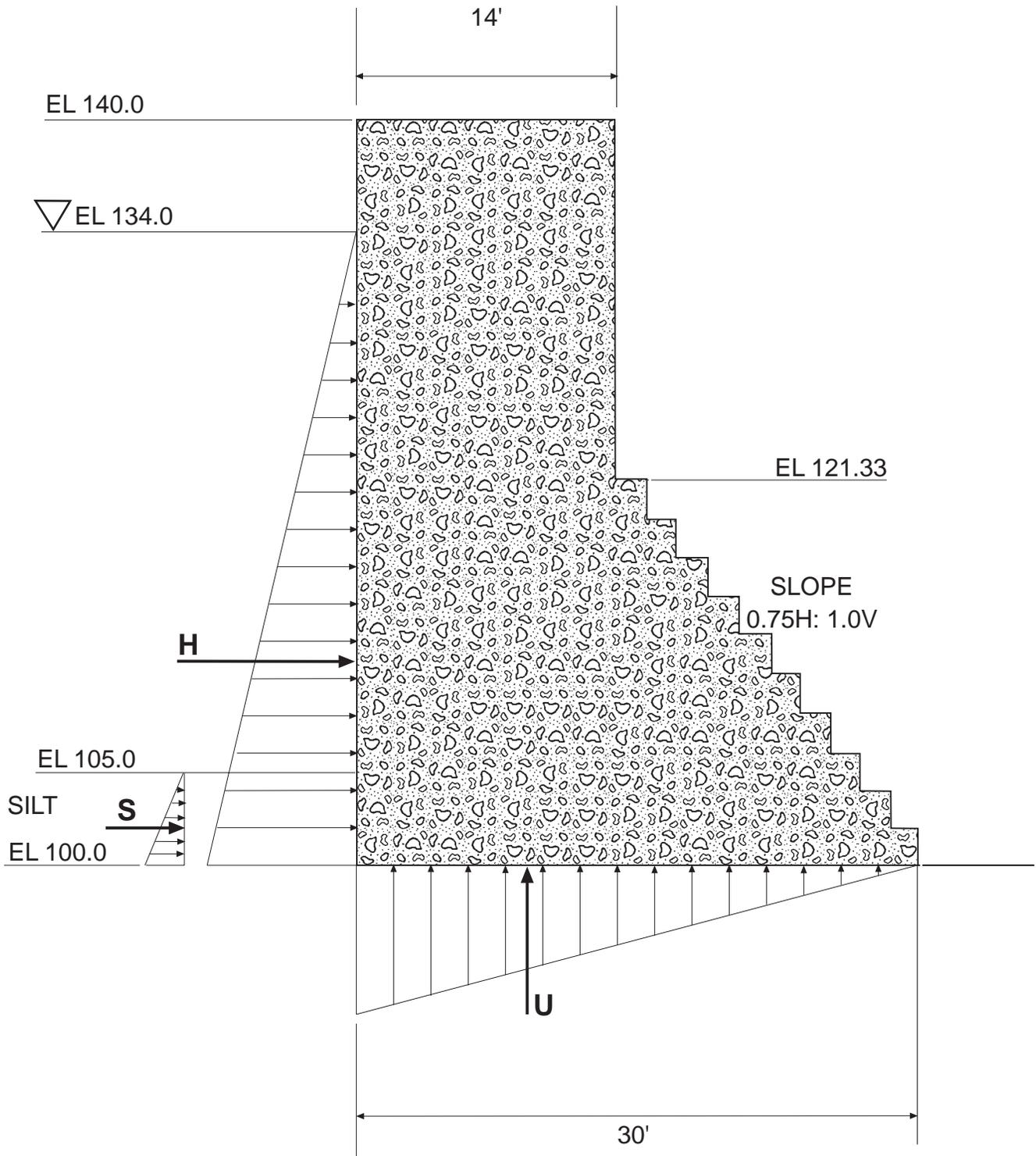
Figure A2. Loading Condition 2 Normal Pool with Seismic Load
