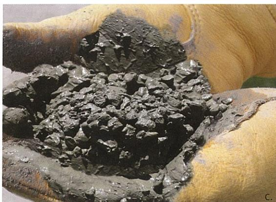
*Figure 5. Samples of pervious concrete with different water contents, formed into a ball: (a) too little water, (b) proper amount of water, and (c) too much water.*
