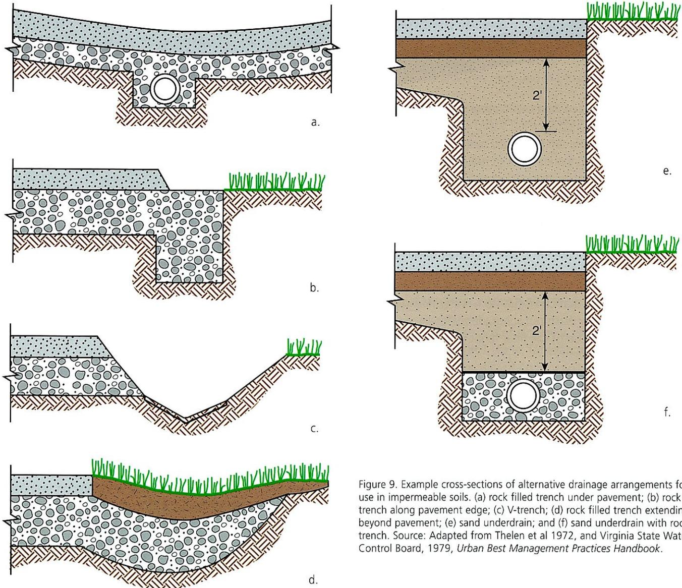
Figure 9. Example cross-sections of alternative drainage arrangements for use in impermeable soils. (a) rock filled trench under pavement; (b) rock trench along pavement edge; (c) V-trench; (d) rock filled trench extending beyond pavement; (e) sand underdrain; and (f) sand underdrain with rock trench. Source: Adapted from Thelen et al 1972, and Virginia State Water Control Board, 1979, *Urban Best Management Practices Handbook*.
