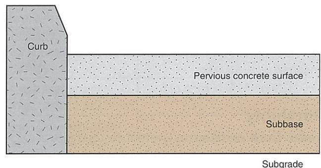
*Figure 3. Typical cross section of pervious concrete pavement. On level subgrades, stormwater storage is provided in the pervious concrete surface layer (15% to 25% voids), the subbase (20% to 40% voids), and above the surface to the height of the curb (100% voids). Adapted from Paine 1990.*
