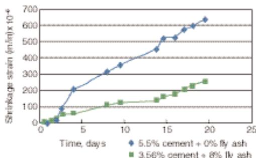
Figure 5-4. Drying shrinkage affected by fly ash, soil #1 (ideal curing, restrained).
