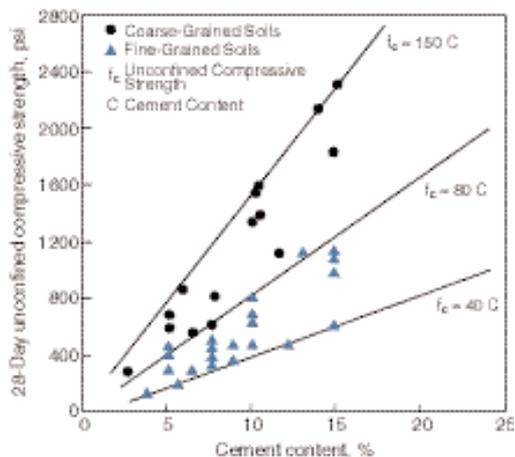
Figure 6-1. Unconfined compressive strength related to cement (adapted from reference 17).
