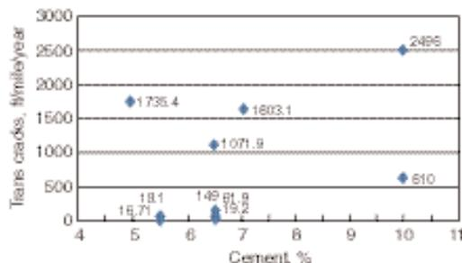
Figure 2-7. Transverse cracks, reflected through the surface, related to cement (Mississippi pavements).
