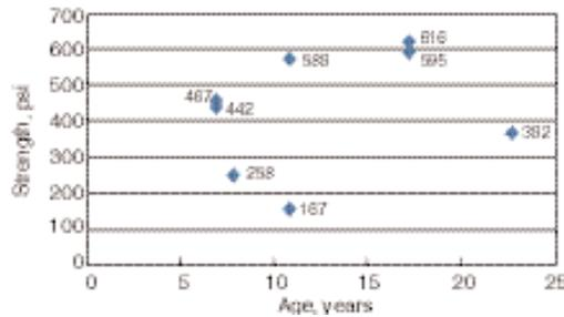
**Figure 3-9. Core strength related to age (LTPP-GPS sections).**
