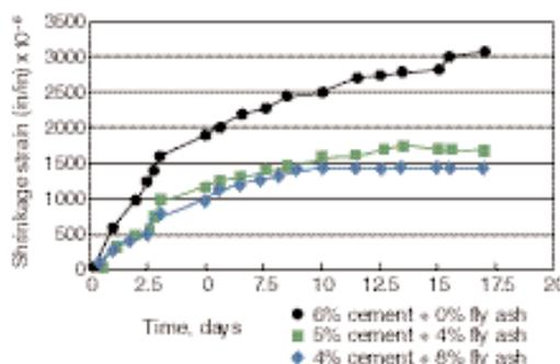
Figure 5-5. Drying shrinkage affected by fly ash, soil #2 (ideal curing, unrestrained).
