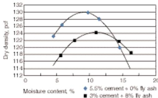
Figure 5-1. Moisture-density relationship with and without fly ash (Soil #1).
