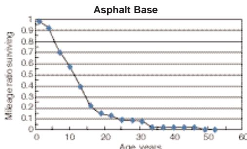
Figure 2-2. Survivor curve for asphalt base pavements. Expected (mean) life = 13.3 years.
