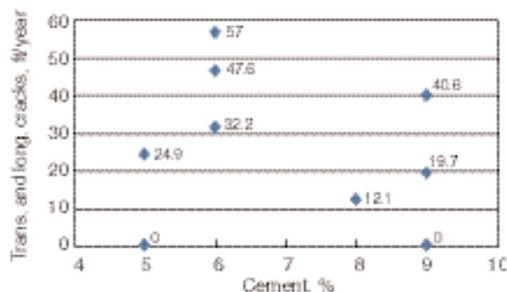
Figure 3-6. Transverse and longitudinal cracks, reflected through the surface, related to cement (LTPP-GPS sections).
