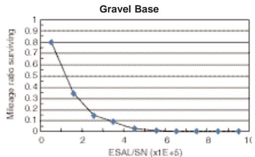
Figure 2-6. Survivor curve for gravel base pavements with respect to ESAL/SN. Expected (mean) ESAL/SN =  $1.2 \times 10^5$
