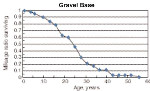
Figure 2-3. Survivor curve for gravel base pavements. Expected (mean) life = 24.4 years.
