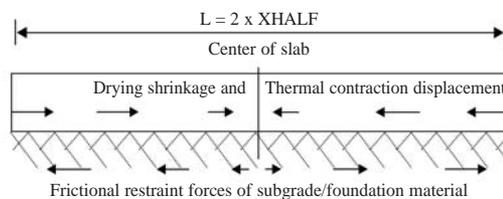
**Figure 4-1. Slab displacement and frictional restraint forces due to drying shrinkage and/or temperature changes (adapted from reference 18).**
