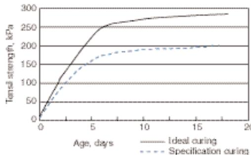
Figure 4-5. Tensile strength-time relationship for soil-cement under different curing conditions (Soil #1).
