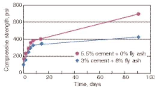
Figure 5-2. Increase in compressive strength with time (Soil #1).
