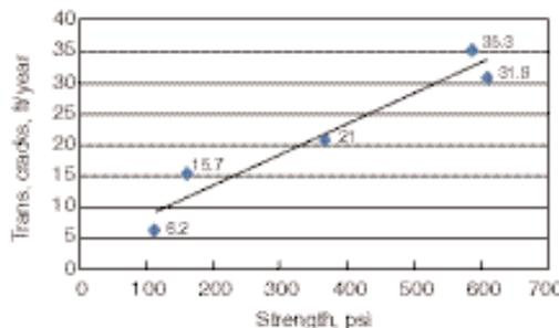
Figure 3-7. Transverse cracks, reflected through the surface, related to strength (LTPP-GPS sections).
