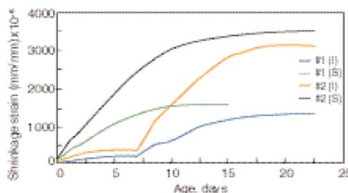
Figure 4-3. Shrinking vs. time for soil-cement (I = Ideal curing, S = Specification curing).
