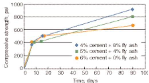
Figure 5-3. Increase in compressive strength with time (Soil #2).
