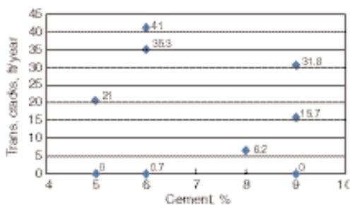
Figure 3-5. Transverse cracks, reflected through the surface, related to cement (LTPP-GPS sections).
