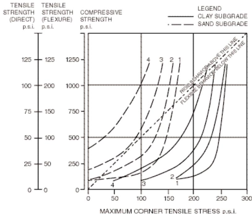
Figure 6-2. Pavement Strength vs. Tensile Stress Due to a Single Wheel Load of 5000 lb on a 6 in. Pavement (Adapted from Reference 32).
