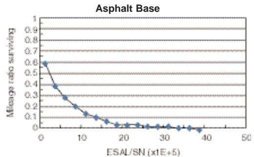
Figure 2-5. Survivor curve for asphalt base pavements with respect to ESAL/SN. Expected (mean) ESAL/SN =  $2.0 \times 10^5$
