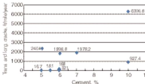
Figure 2-8. Transverse cracks, reflected through the surface, related to cement (Mississippi pavements).
