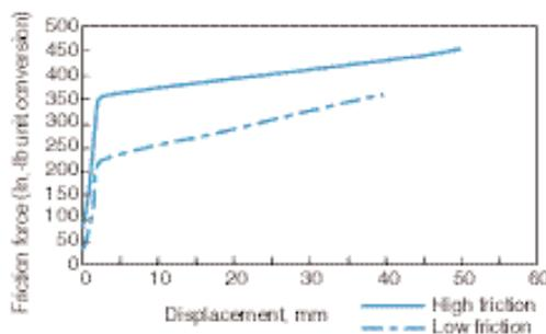
Figure 4-2. Friction force between soil-cement base and subgrade vs. displacement (adapted partly from reference 18).
