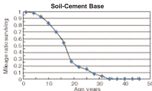
Figure 2-1. Survivor curve for soil-cement base pavements. Expected (mean) life = 17.1 years.
