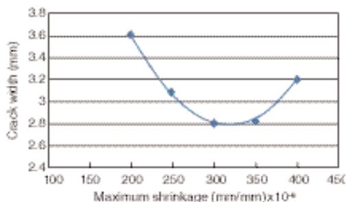
Figure 6-3. Variation of crack width with shrinkage (restrained) of base (coarse-grained soil).
