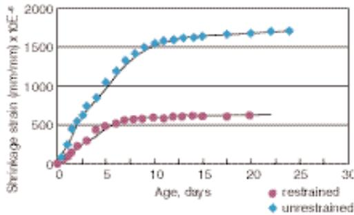
Figure 4-4. Shrinkage strain vs. time for soil-cement (Soil #1, specification chart).
