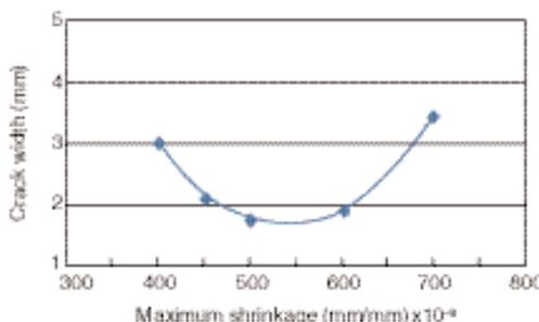
Figure 6-4. Variation of crack width with shrinkage (restrained) of base (fine-grained soil).
