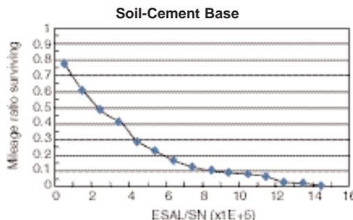
Figure 2-4. Survivor curve for soil-cement base pavements with respect to ESAL/SN. Expected (mean) ESAL/SN =  $3.3 \times 10^5$
