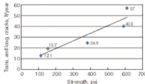
Figure 3-8. Transverse and longitudinal cracks, reflected through the surface, related to strength (LTPP-GPS sections).
