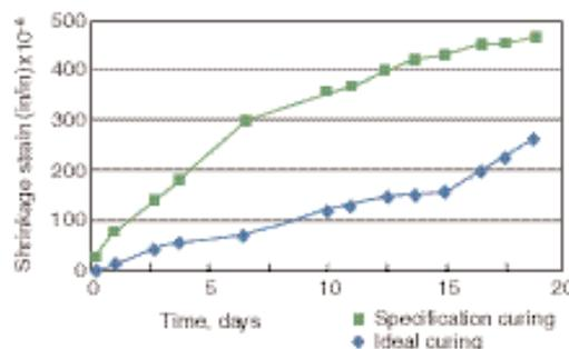
Figure 5-6. Drying shrinkage affected by curing conditions, soil #1.
