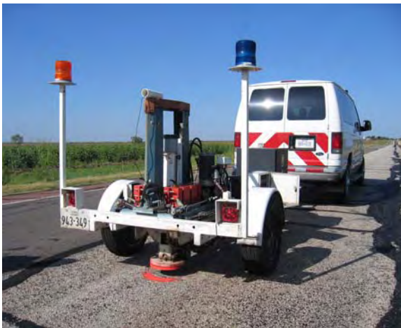
Figure 25. Falling weight deflectometer.
