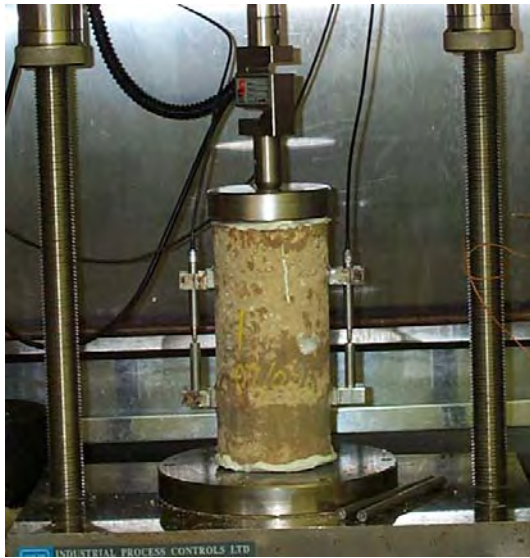
Figure 5. Setup of LVDTs in dynamic modulus test.
