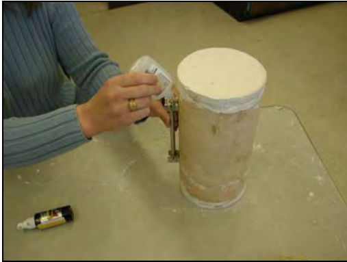
16c) Gluing LVDT Attachments to Sample
