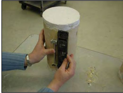
16b) Leveling the LVDT Attachments
