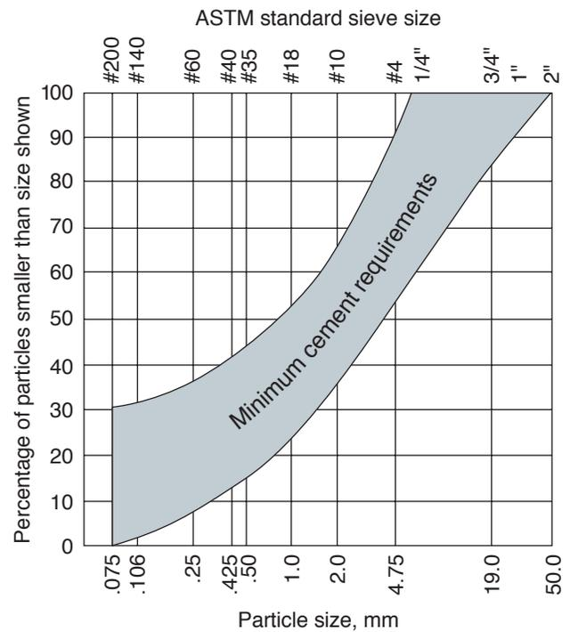
Figure 2.1. Aggregate gradation band for minimum cement requirements.
