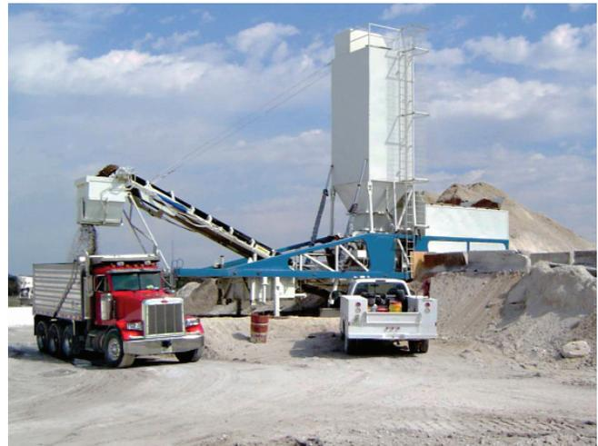
*Figure 3.1. Mixing CTB in a continuous-flow-type pugmill.*
