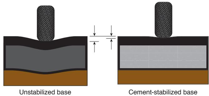
Figure 1.4. Rutting can occur in the surface, base, and subgrade of unstabilized bases due to repeated wheel loading. Cement-stabilized bases resist consolidation and movement, thus virtually eliminating rutting in all layers but the asphalt surface.
