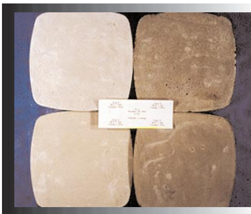
Fig. 2. All samples (L): 1 day old, wet storage, finished surface. Top left: w/c = 0.5, Type I cement. Bottom left: w/c = 0.8, Type I cement. Top right: w/c = 0.5, Type V cement. Bottom right: w/c = 0.8, Type V cement. (68348)
