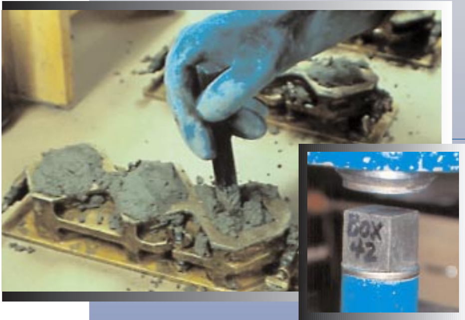
Fig. 1. 50-mm (2-in.) mortar cubes are cast (left) and crushed (right) to determine strength characteristics of cement. (69128)(69124)
