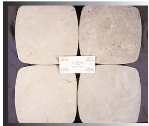
Fig. 3. All samples (R): 90 days old, wet storage, finished surface. Top left: w/c = 0.5, Type I cement. Bottom left: w/c = 0.8, Type I cement. Top right: w/c = 0.5, Type V cement. Bottom right: w/c = 0.8, Type V cement. (68349)
